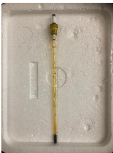
Figure IV-13. A J.-Young tube that being used to set up the polymerization reaction.
