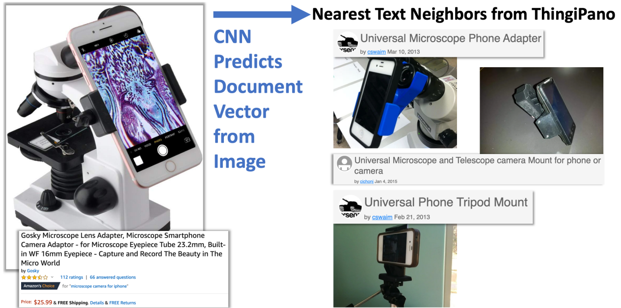
Figure 7.7: A Multi-Modal retrieval example utilizing a deep learning model trained with ThingiPano images and metadata. Reprinted with Permission from “ ThingiPano: A Large-Scale Dataset of 3D Printing Metadata, Images, and Panoramic Renderings for Exploring Design Reuse ”[1]
