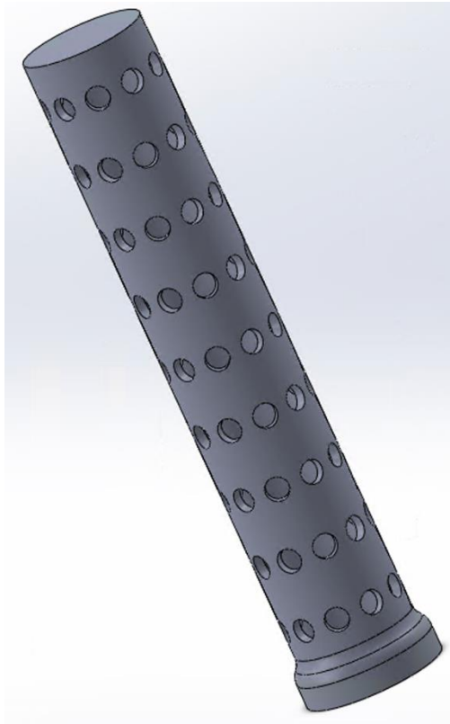
Figure 3.23 Example injector head with showerhead configuration. The outer diameter of the injector is 1.5” and the overall length is approximately 5.00”.
