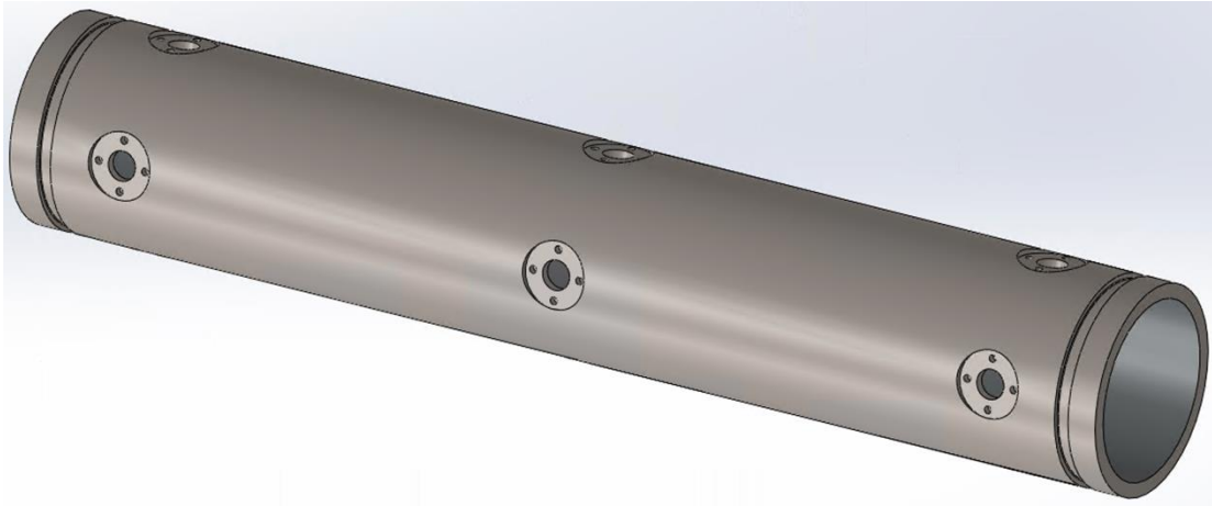
Figure 3.2 View of driven tubing section. Ports are shown with spacing of 16". Grooves on each end accommodate the flanges.
