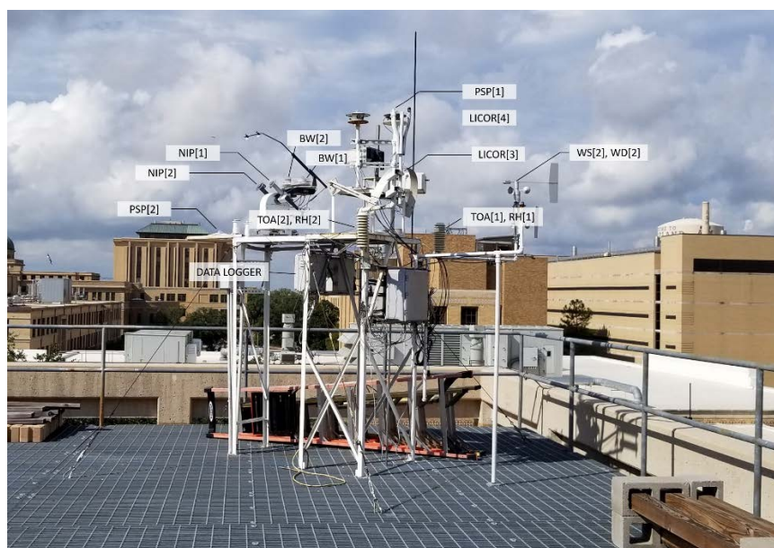
Figure 64. Exterior View of the Solar Test Bench
