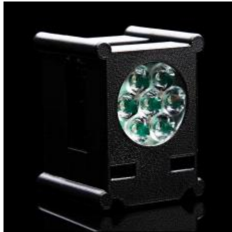
Figure 24. High power LED lamps used to illuminate the LA.
