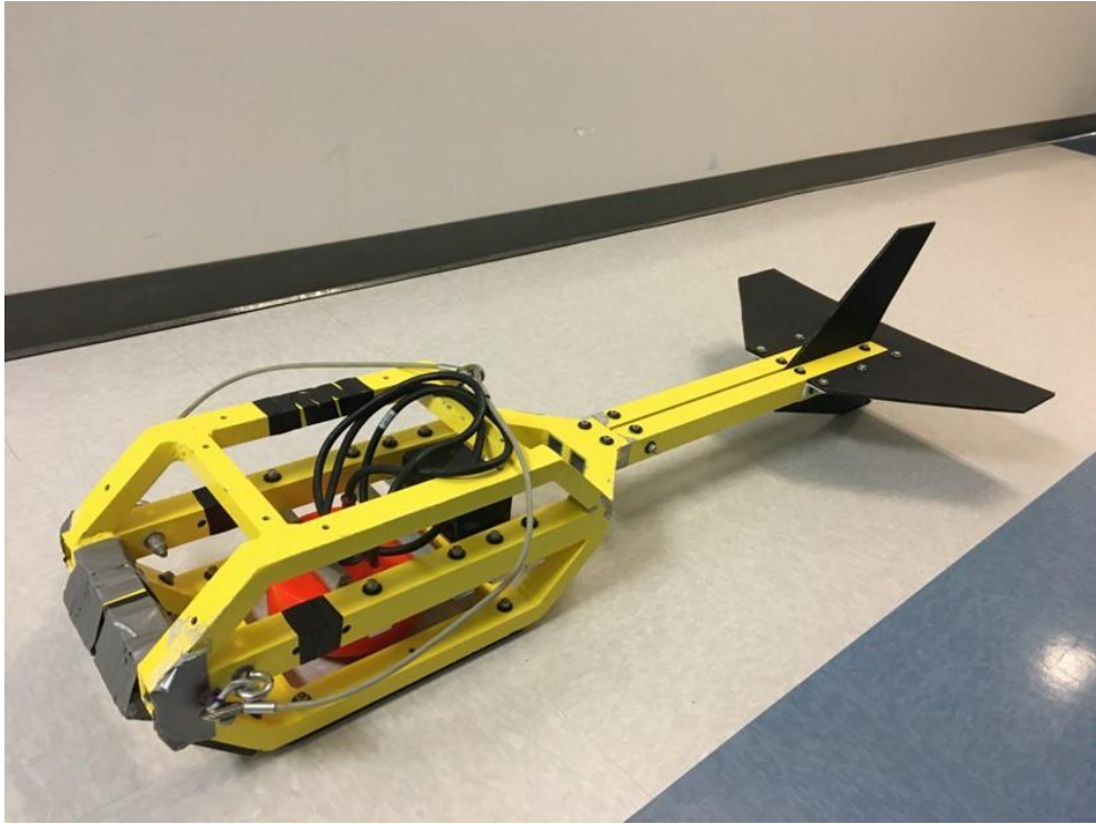
Fig. 2: Tow body for the echo sounder transducer (orange cylinder at frame center).
