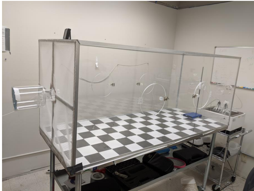
Figure 3.2 – Dual-Port Olfactometer. Release cage is on left, while odor ports are on right.
