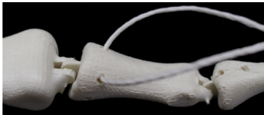
Figure 15: Canine middle phalanx demonstrating attachment point for a muscle built into 3D printed model
