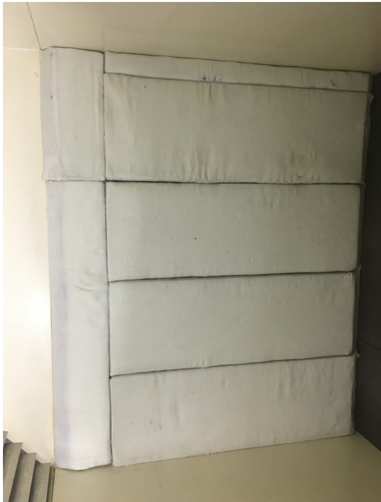
Figure 5.10: Acoustic panels mounted to the settling chamber by senior design team.
