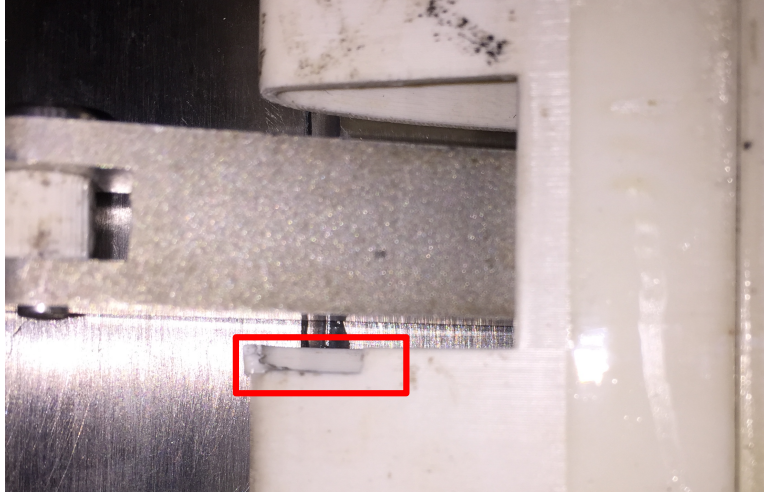
Figure 5.26: Missing material (highlighted in red) on the leading edge of the wing. This geometric discontinuity was the cause of high decibel tonal noise.
