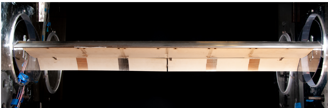
Figure 2.2: Experimental setup of CRM wing treated with SMA SCF.
