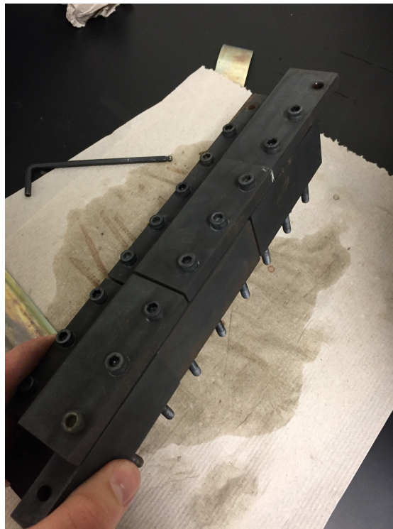
Figure 2.3: Steel mold used to geometrically configure the SMA SCF.
