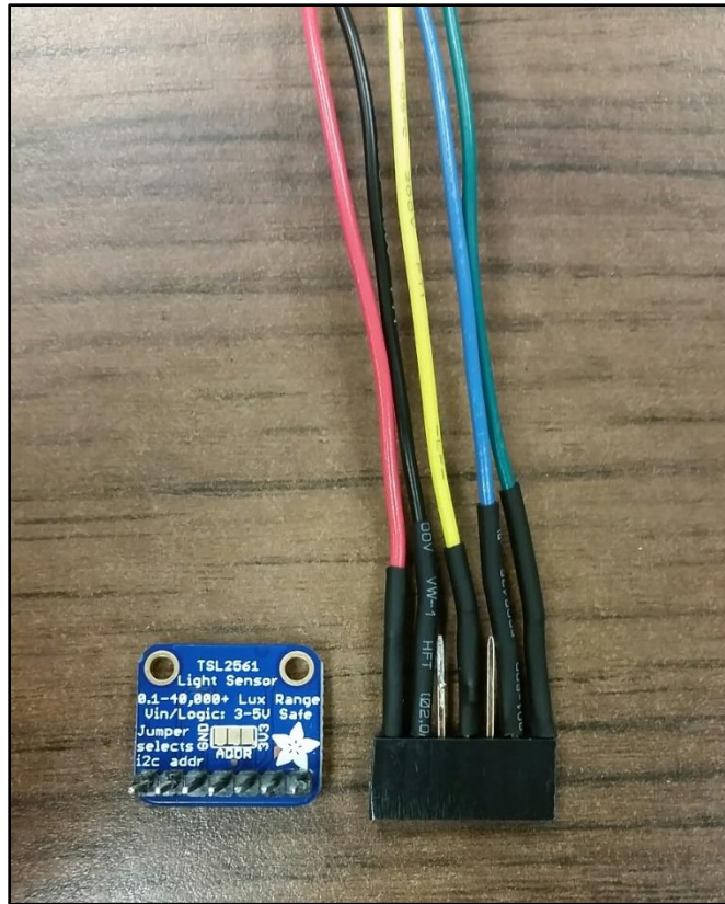
Figure 3. The TSL-2561 digital lux sensor with the stacking header that attaches to the respective pins on the OS board.
