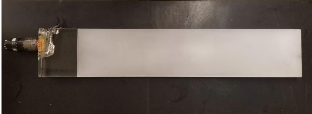
Figure 20. The PVT detector remained fully opaque at room temperature and RH as a result of significant damage from microfractures following multiple temperature cycles in the ORNL environmental chamber.
