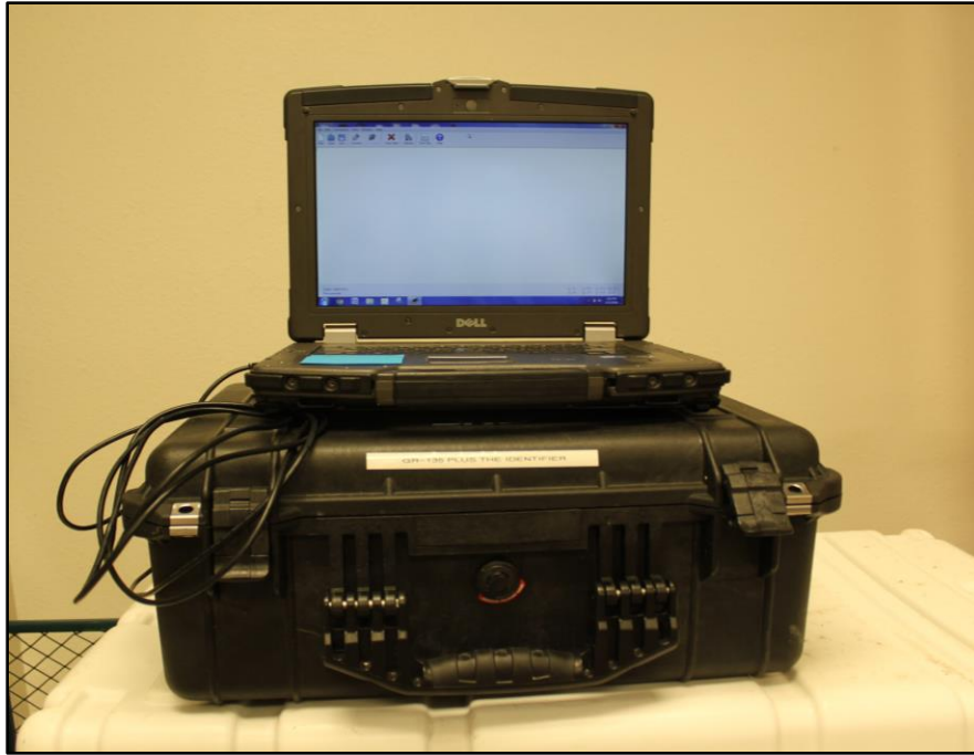
Figure 8. Arrangement of the OMS data acquisition testing environment showing the protective case containing the PVT detectors with onboard OMS and Arduino Mega microcontroller (unseen), and the testing laptop with USB running between computer and microcontroller.
