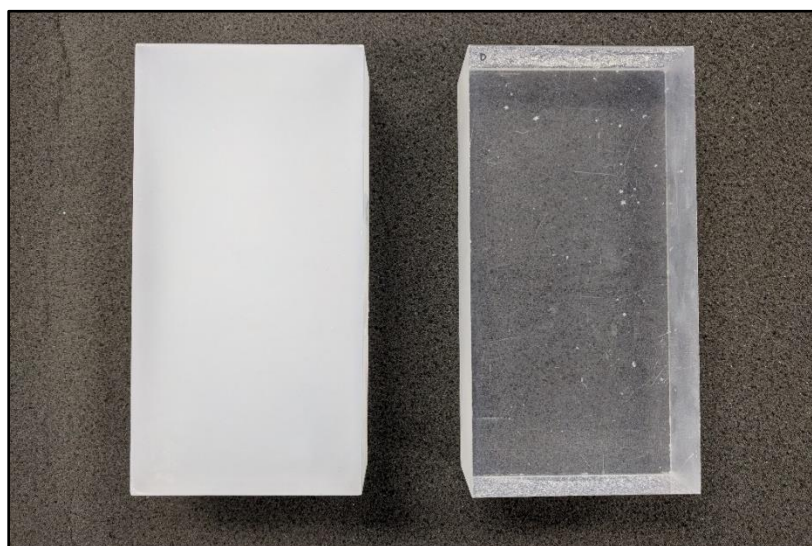
Figure 7. Two PVT detectors of size 14.92 cm x 7.62 cm x 3.81 cm, one fully opaque from high temperature and high humidity soak and 24 hours of low temperature and RH (left), and the other transparent at RT and RH (right).
