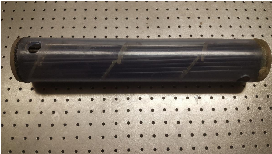
Figure 32. Tri-section Helical Baffle Heat Exchanger
