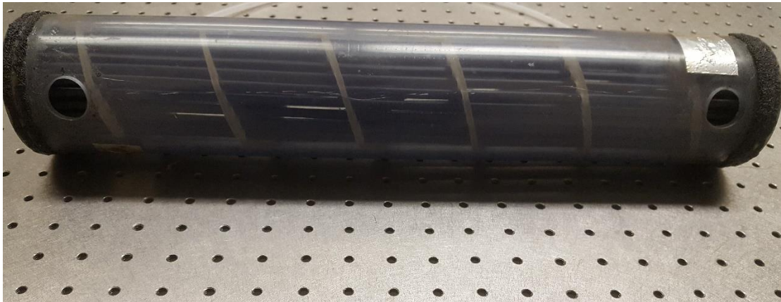
Figure 30. Continuous Helical Baffle Heat Exchanger
