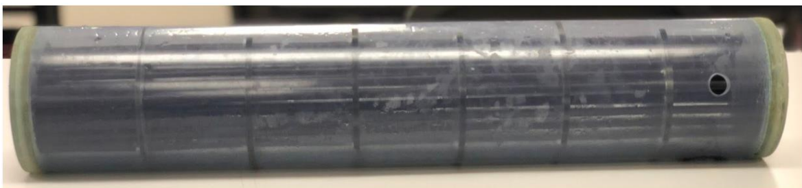
Figure 28. Heat Exchanger with segmental baffles
