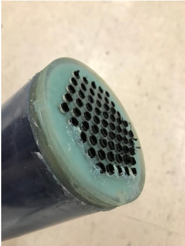
Figure 26. Sealed manifold with tubing
