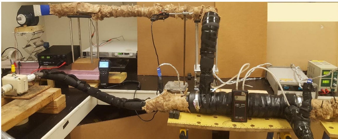
Figure 22. Arrangement of physical experimental set up for single phase heat transfer tests
