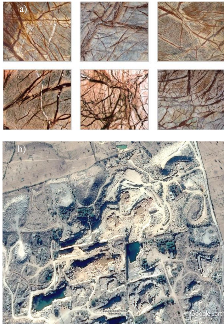
Figure 2-3 a) Examples of rock slabs from Bidasar with bifurcating, hydraulic injection veins. Image dimensions about 1 square meter (courtesy Dewan Group). b) Satellite image of quarry near Bidasar, Rajasthan, India (roads for scale). North is down in above image (Google Earth composite of 16 Dec 2015).
