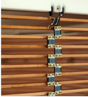
Figure 2.14: This shows the voltage divider which connected to the field-shaping rings and helped to maintain a vertical drift field in the fiducial volume. This upper portion shows how it connected to the gate grid and shows how the resistor pairs were mounted on Cirlex® board. Photograph reprinted from [59].
