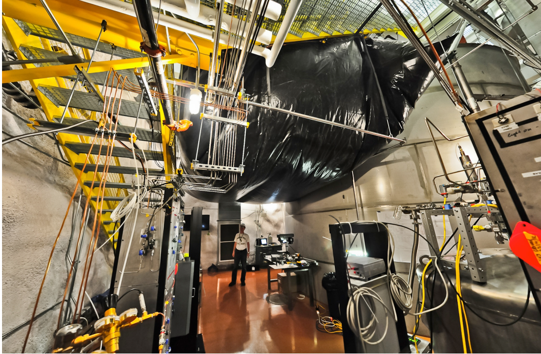
Figure 2.10: This photograph shows a test of the recovery balloon underground. The 70 m 3 volume balloon could hold 370 kg of xenon at standard temperature and pressure which would inflate the balloon to 95% of its capacity. Photograph reprinted from [18].
