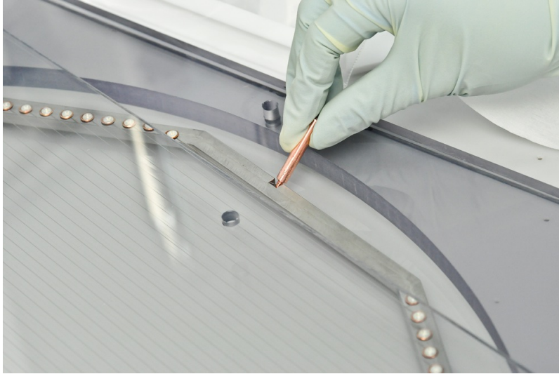
Figure 2.12: This photograph shows a close view of the cathode grid which had 0.5 mm spacing. The copper cylinder shown served as part of the high voltage connection. Photograph reprinted from [59].
