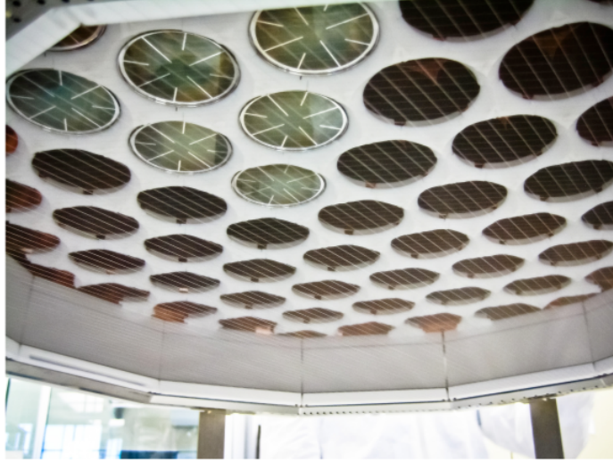
Figure 2.7: This photograph shows PMTs being installed into the top array in LUX. Note that the area between the PMTs is filled by a PTFE surface. Figure reprinted from [18].
