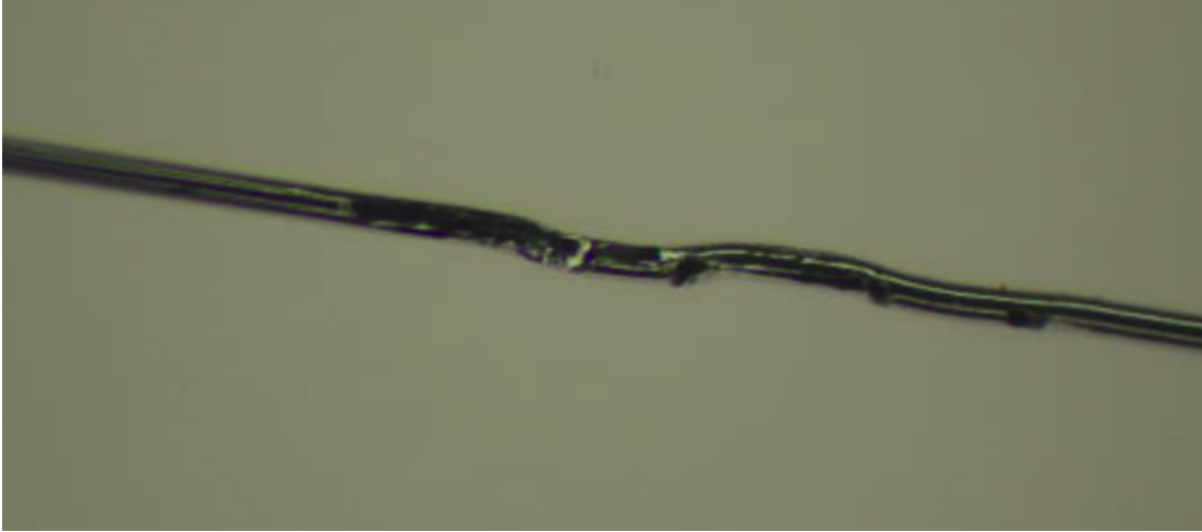
Figure 2.16: The above photograph shows a damaged grid wire discovered during the LUX post-mortem investigation of the grids. The image appears to show a wire that had been heavily burnt and deformed, possibly having resulted from the conditioning campaign.
