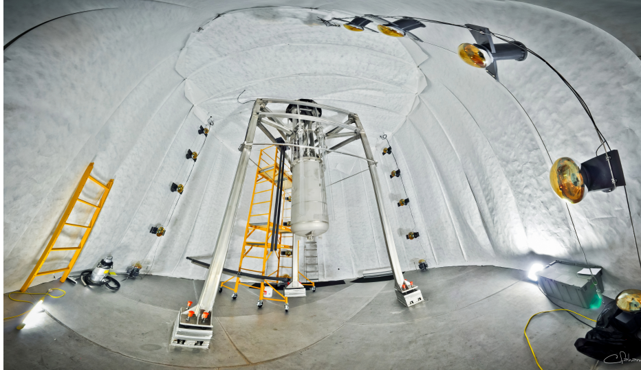
Figure 2.23: This picture came from inside the LUX water tank muon veto system prior to being filled with water. Minimum water shielding was 2.75 m above, 3.5 m along its circumference, and 1.2 m below. It contained 270,000 L of ultra-pure water. Included in the picture are some of the Hamamatsu R7081 10 in PMTs for detection of Cherenkov radiation, which were in operation for Run04. Picture reprinted from [18].
