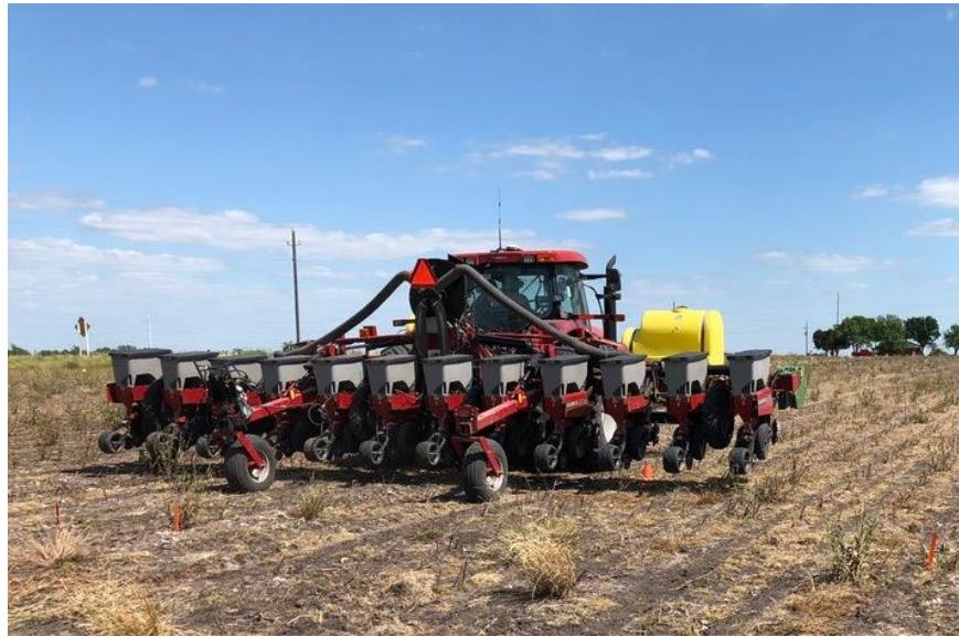
Figure 2.7 CASE IH 1230 12-row Early Riser planter used in the experiment.
