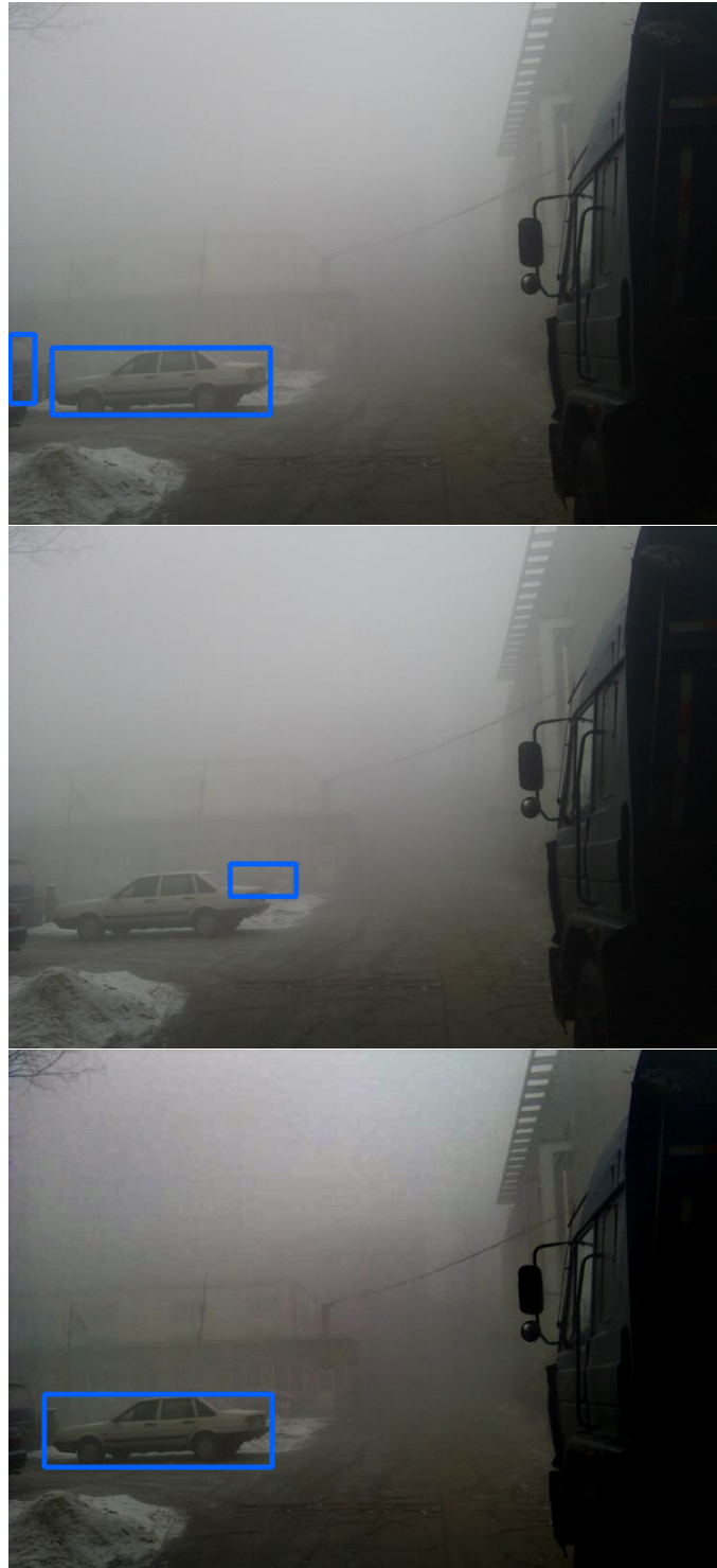
Figure 3.10: Image Enhancement Corrects Bounding Box Position in Detection. The top row displays the raw hazy image annotated with ground truth bounding boxes; the middle row displays raw image with bounding boxes detected by pre-trained Mask R-CNN; the bottom row displays image enhanced by pre-trained MSCNN with bounding boxes detected by pre-trained Mask R-CNN.
