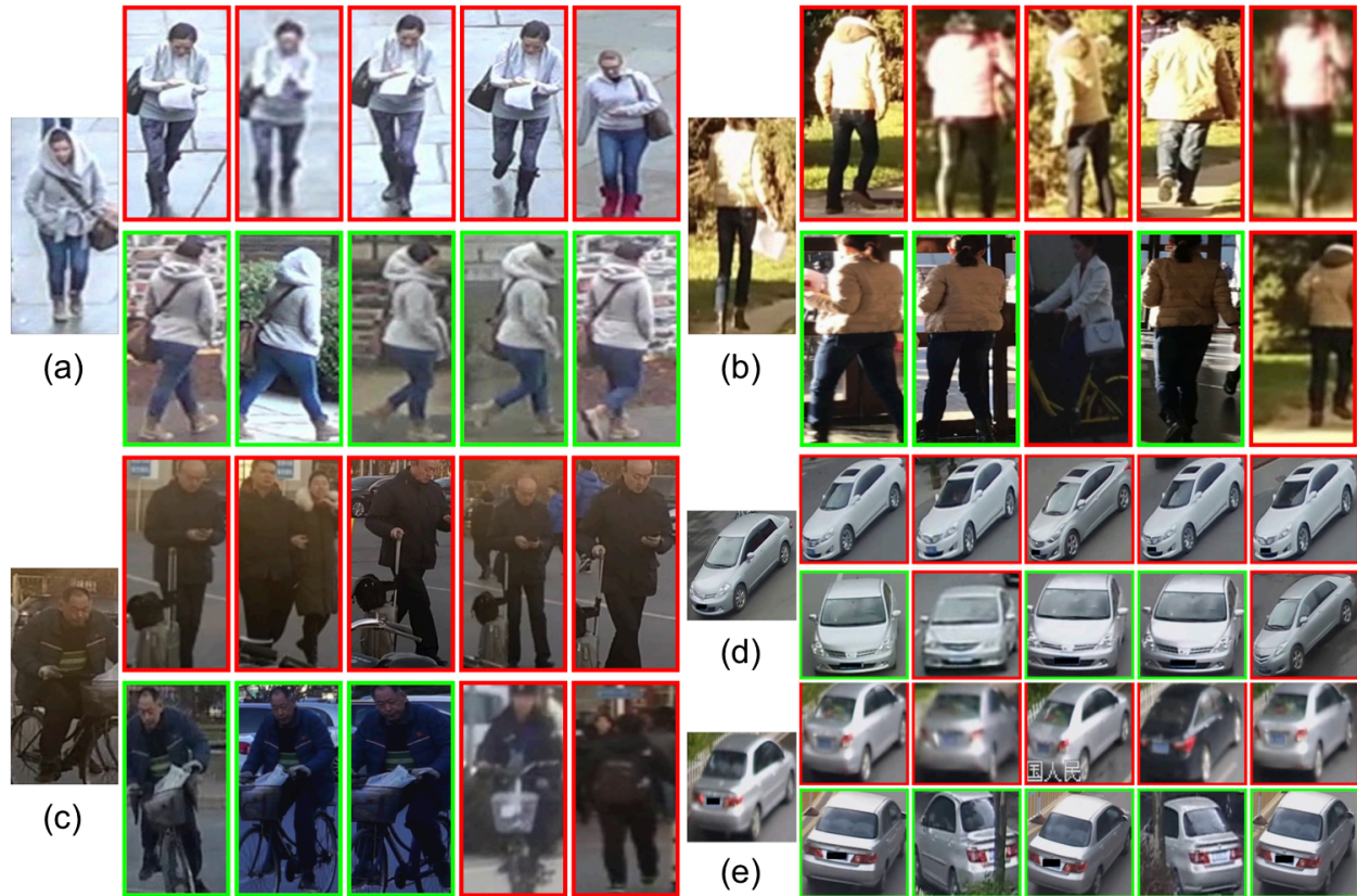
Figure 6.3: Comparison of Retrieval Results w/o ADIN. Retrieval results on the DukeMTMC-ReID (a), MSMT17 (b, c), and VeRi-776 (d, e). The leftmost image in each panel is a query image. For the five columns in each panel, the top row shows top-5 retrieval results using a vanilla ResNet50 model [184], and the bottom row shows top-5 results using ResNet50 adopted with ADIN framework. Green boxes mark the correct matches, while red boxes denote the wrong matches. The vanilla ResNet50 tend to retrieve images with similar nuisances (illumination, view-points, scene backgrounds, etc.), while ADIN successfully eliminates nuisances and leads to more robust matching under drastic visual appearance changes.
