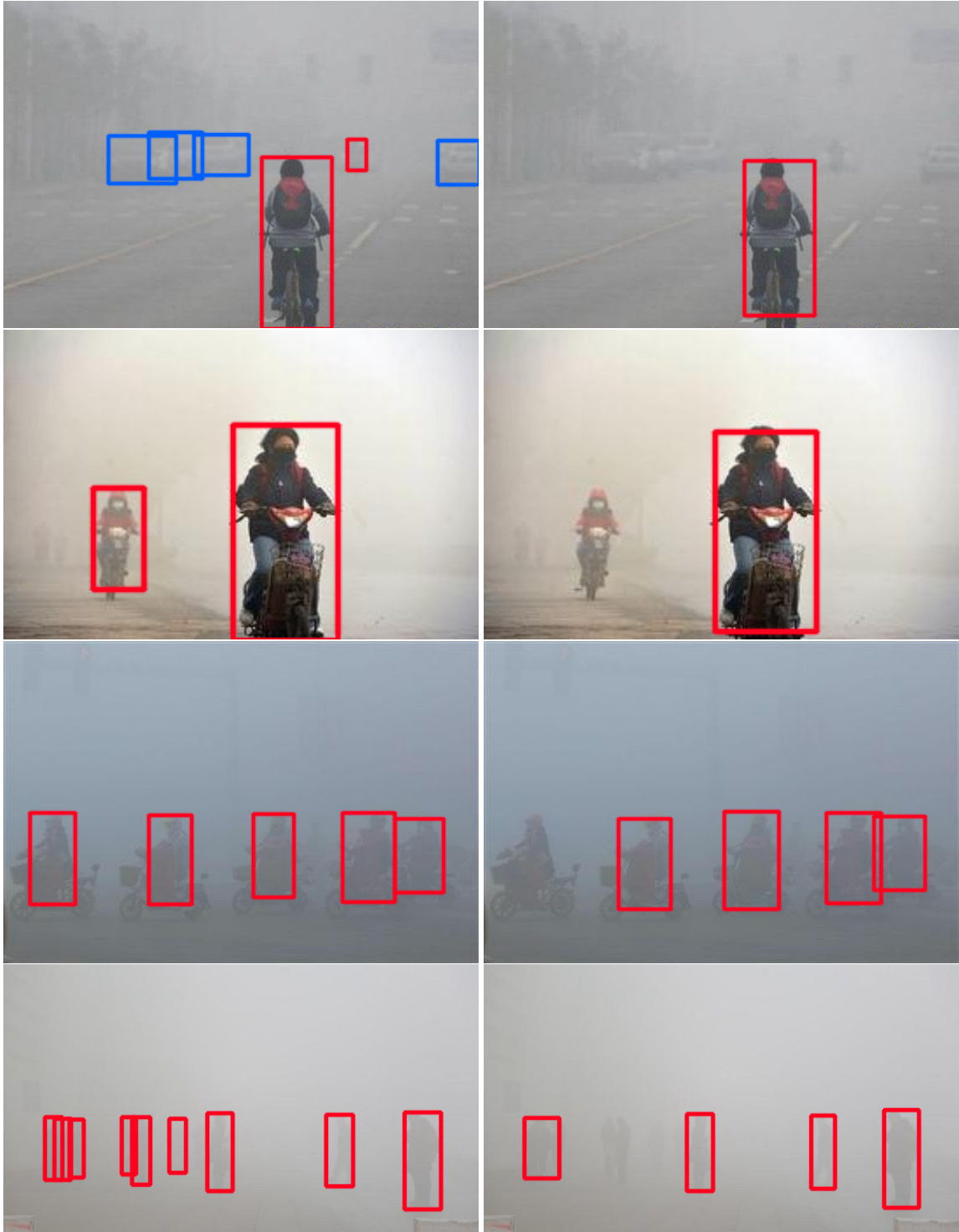
Figure 3.1: Failure Case of Object Detection in Poor Visibility Environments. The left column displays the raw hazy image annotated with ground truth bounding boxes; the right column displays raw image with bounding boxes detected by pre-trained Mask R-CNN.
