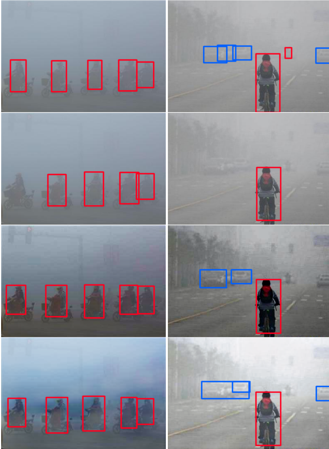
Figure 3.7: Image Enhancement Benefits Detection Quantitatively. The top row displays the raw hazy image annotated with ground truth bounding boxes; the second row displays raw image with bounding boxes detected by pre-trained Mask R-CNN; the third and fourth row displays image enhanced by pre-trained MSCNN and DCPDN with bounding boxes detected by pre-trained Mask R-CNN.
