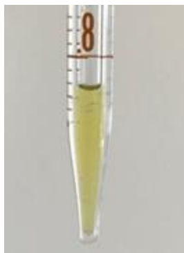
Figure 65 – Color of produced oil (lighter than original oil) from the CH 4 experiment.
