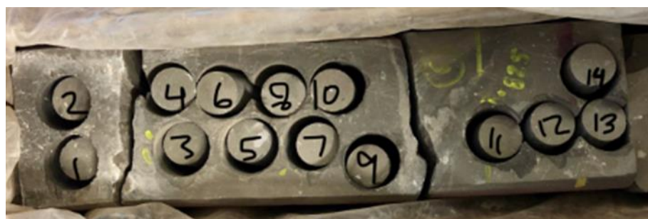
Figure 58 – Core Plugs cut from the Wolfcamp A formation in Martin County, TX.
