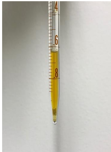
Figure 75 – Color of produced oil (darker than all other gas experiments) from the CO 2 test.
