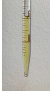
Figure 71 – Color of produced oil (slightly darker than other produced oil) from the enriched gas test.
