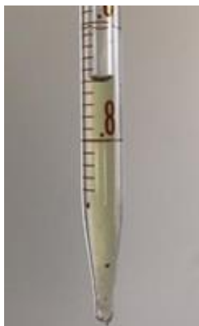
Figure 68 – Color of produced oil (lighter than original oil) from the mixture of 85% CH 4 and 15% C 2 H 6 experiment.
