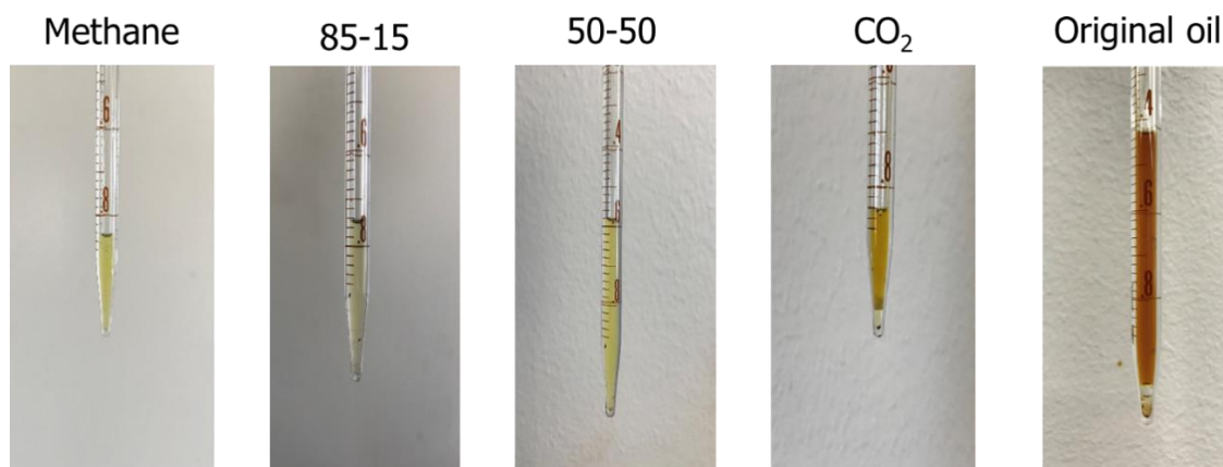
Figure 90 – The color of produced oil from all four gas Huff-n-Puff experiments. Gas 85/15 refers to the gas mixture of 85% CH 4 and 15% C 2 H 6 , Gas 50/50 refers to enriched gas (50% CH 4 and 50% C 2 H 6 ), and original Wolfcamp oil.
