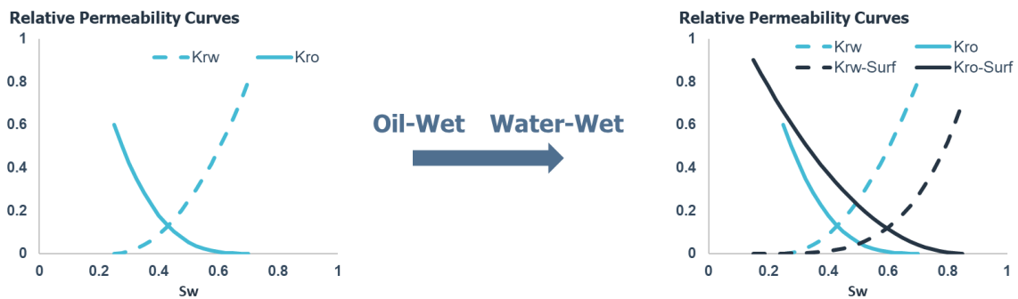
Figure 9 – The change of relative permeability as the wettability altered from oil-wet to water-wet.
