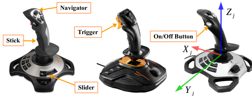
Figure 7.2: General Purpose Joysticks and Common Features
