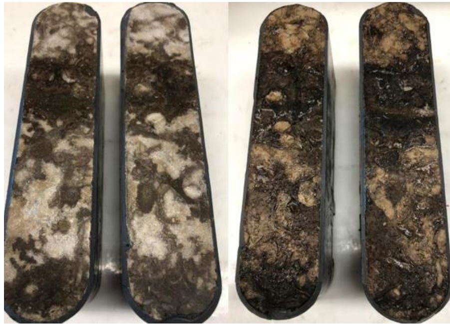
Figure 3-22: Test 15 before acidizing (left) and after acidizing (right).
