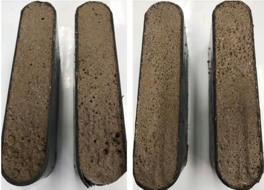
Figure 3-4: Test 1 (left) and Test 3 (right) fracture surfaces after acidizing.
