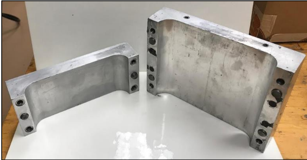
Figure 2-5: Left mold (Acidizing sample preparation) and right mold (Fracture conductivity sample preparation).
