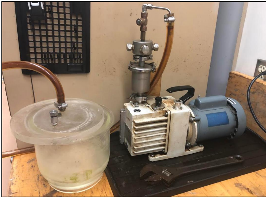
Figure 2-2: Vacuum pump used to saturate core samples.
