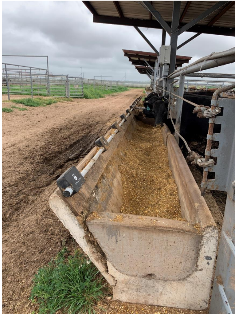
Figure 3.3 Ultra-wideband RFID receivers used to capture electronic feeding behavior in trial 1.
