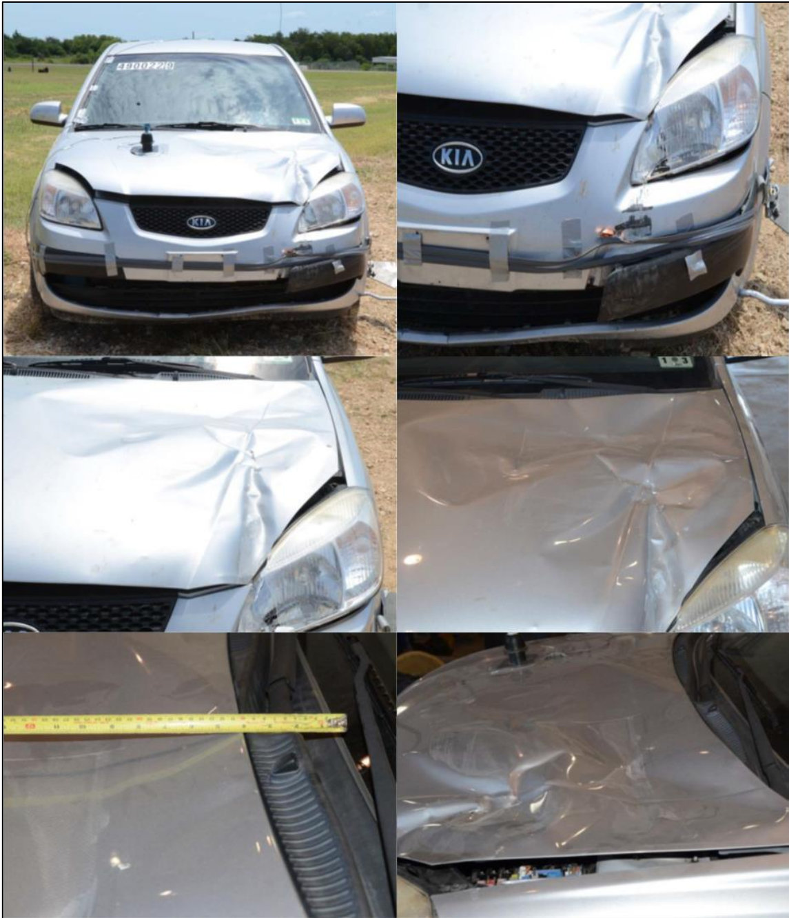
Figure 19. Vehicle After the MASH 3-61 Test (Reprinted from Silvestri et al., 2013)
