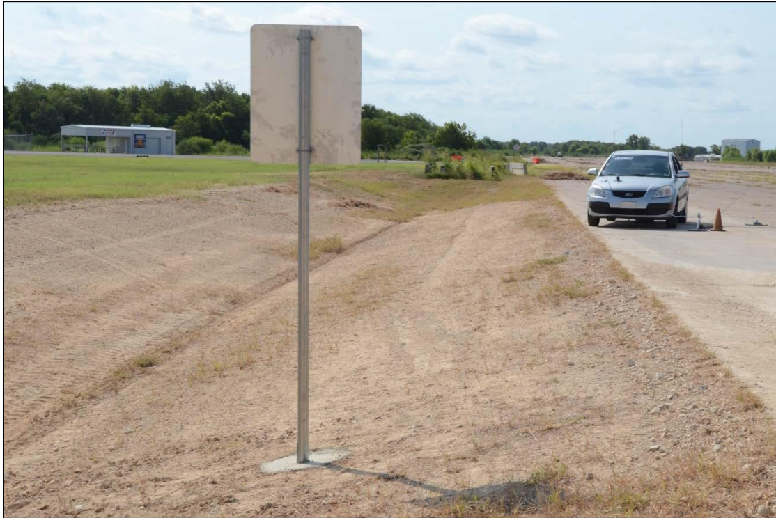
Figure 18. Vehicle and Test Article for Slope Test (Reprinted from Silvestri et al., 2013)
