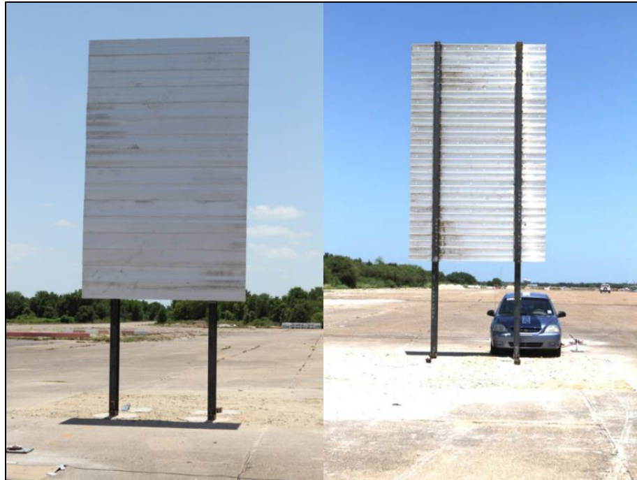
Figure 12. TxDOT W8x18 – 16-ft x 10-ft Large Sign Support System (Reprinted from Silvestri et al., 2011)
