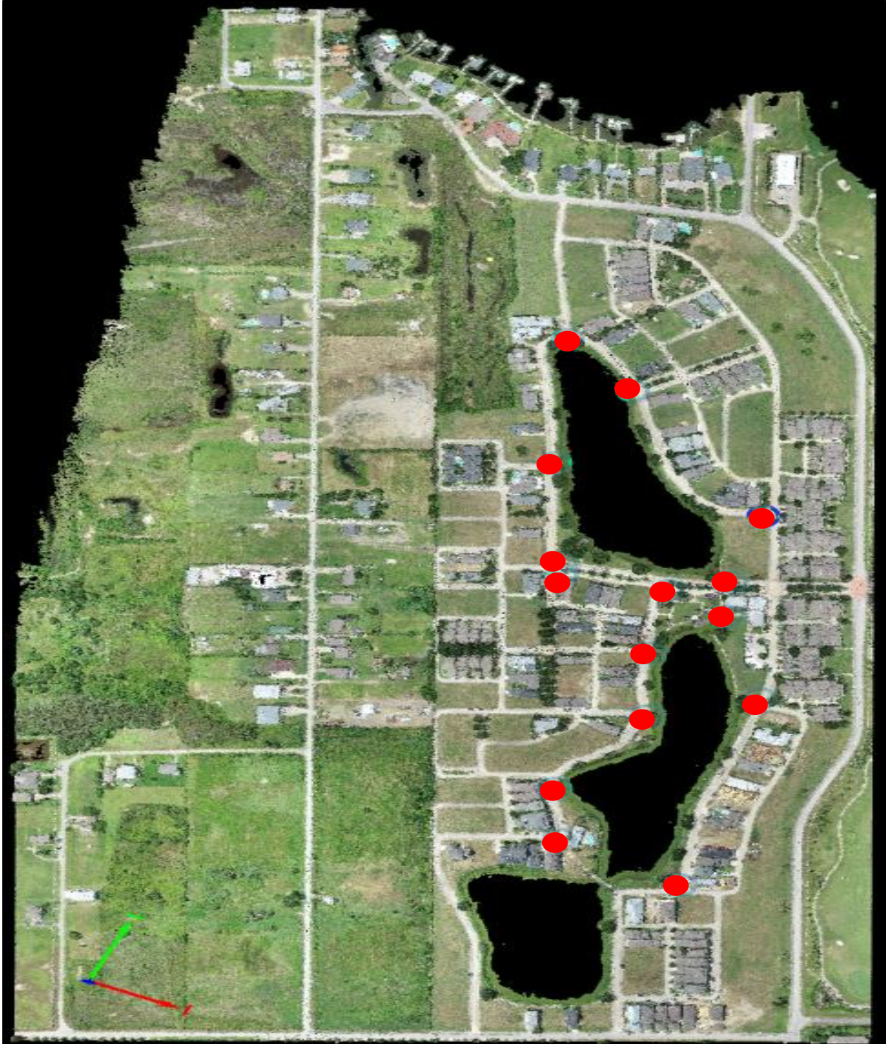
Figure 12: Evia DPC and 3D model. Red dots represent GCPs (processed in Pix4D).
