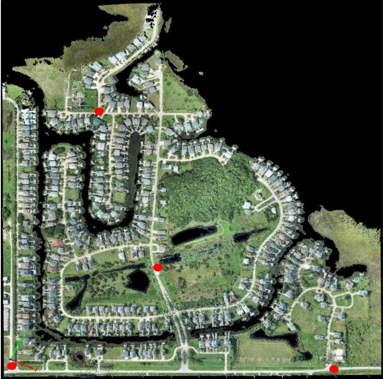
Figure 9: Lafitte's Cove DPC and 3D mesh sections merged. Red dots represent GCPs (processed in Pix4D).
