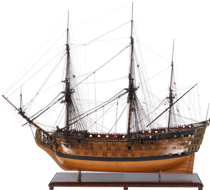
Figure 23. A model of Victory (1737) depicting both a sprit topmast and a jibboom with associated headsails. (Royal Museums Greenwich, object ID SLR0449).
