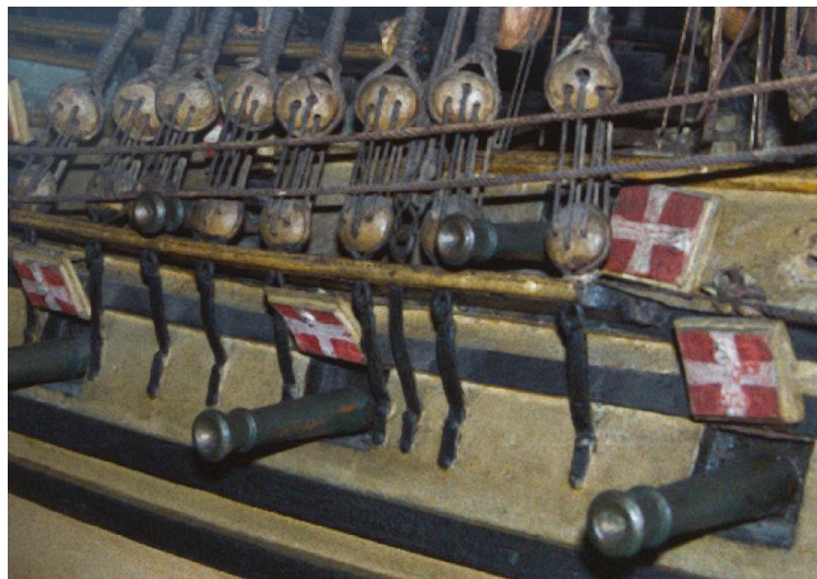
Figure 7. The main channels of the Danish Church model (ca. 1680) showing chainplates constructed from a single iron bar. (Reprinted from Corder 2007, fig. 27).
