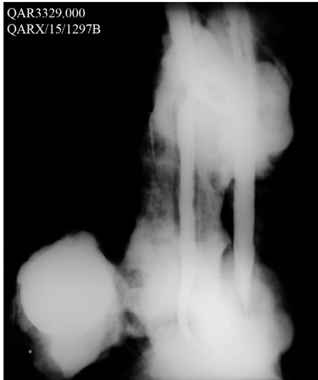
Figure 6. An x-ray of 3329.000, a deadeye strap and chainplate assembly, clearly showing the chain links of the chainplate. (Image courtesy of the Queen Anne's Revenge Conservation Laboratory, Department of Natural and Cultural Resources, North Carolina).
