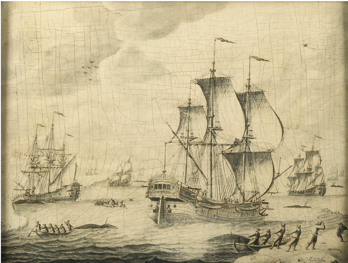
Figure 18. Grisaille on panel by Roelof van Salm, dated 1705. The vessel in the foreground is depicted with a jackstaff and a jibboom. (Royal Museums Greenwich, object ID BHC0939)
