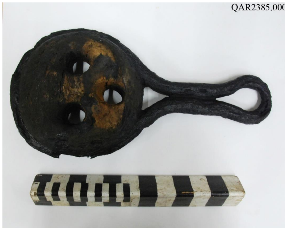
Figure 4. QAR 2385.000, the sole deadeye conserved to date from Queen Anne's Revenge . (Image courtesy of the Queen Anne's Revenge Conservation Laboratory, Department of Natural and Cultural Resources, North Carolina).
