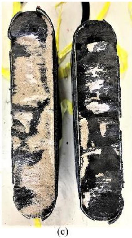
Figure 32. Images of the proppant distribution on the fracture surfaces after the Meramec cores were tested: (a) Sample No. 1 with provided proppant; (b) Sample No. 2 with provided proppant; (c) Sample No. 3 with created proppant; (d) Sample No. 4 with created proppant.
