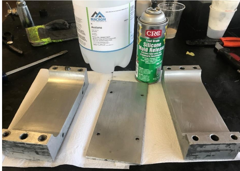
Figure 16. The mold with the chemicals used to prepare it for the sample and epoxy resin.
