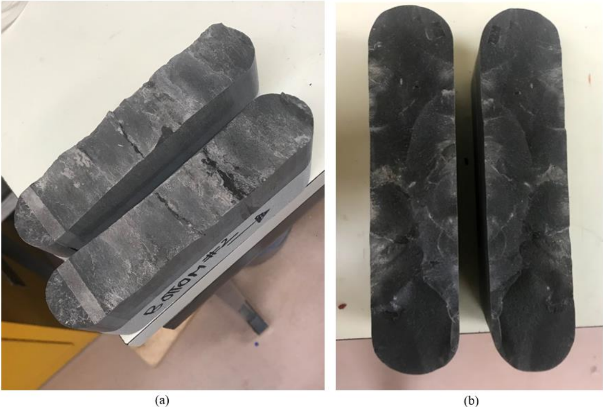
Figure 9. The surfaces created by Kochurek Industries using the tension method: (a) fracture surfaces of a Meramec shale sample (Sample No. 2); (b) fracture surfaces of an Eagle Ford shale sample (Sample No.5).
