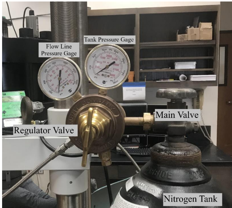
Figure 25. The gages and valves connected the nitrogen tank.
