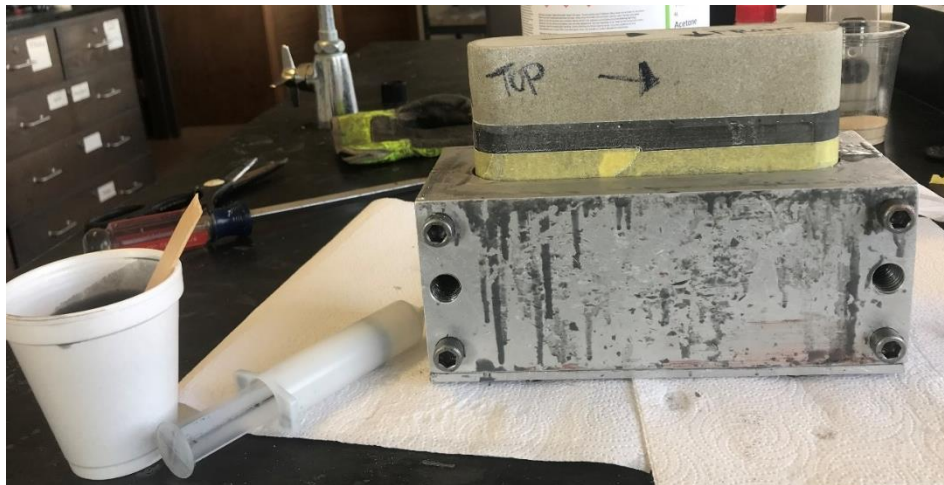
Figure 17. The mold with the sample centered inside with the application syringe and epoxy resin mix.
