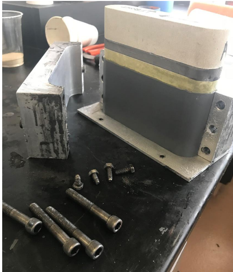
Figure 18. The sample in the mold after curing in the oven for 2 hours.
