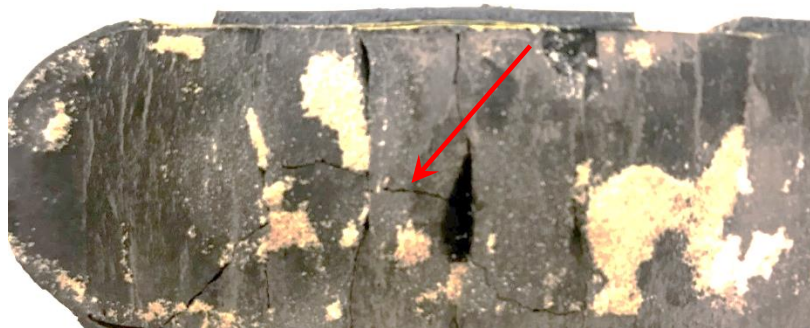
Figure 30. Indicated with the red arrow, the fracture that formed in the fracture surface after Sample No. 2 was tested.
