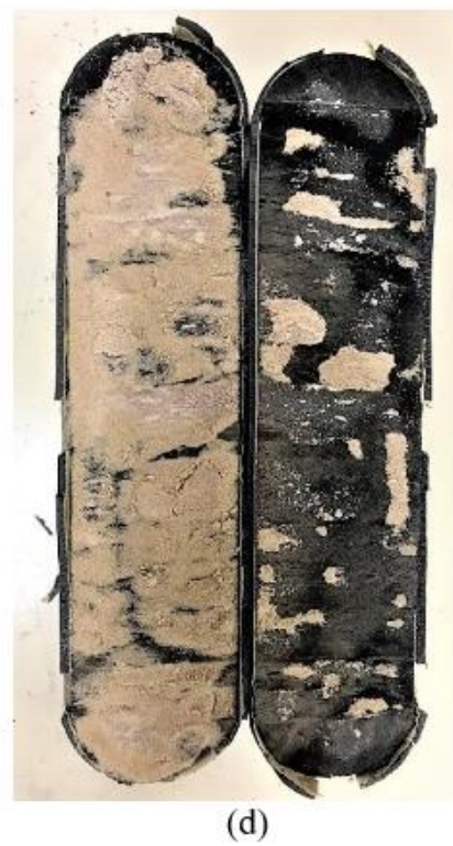
Figure 32. Images of the proppant distribution on the fracture surfaces after the Meramec cores were tested: (a) Sample No. 1 with provided proppant; (b) Sample No. 2 with provided proppant; (c) Sample No. 3 with created proppant; (d) Sample No. 4 with created proppant.
