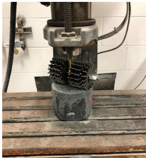
Figure 3.5. 2-3/8 in. (60 mm) Dressing Wheels with Specimen for ASTM C944 Testing
