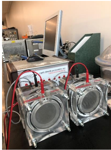
(a) Rapid Chloride Penetration Equipment
