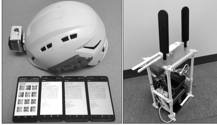
Figure 5.9: A test platform for R-MStorm that consists of a helmet camera, four Android phones and a wireless manpack.
