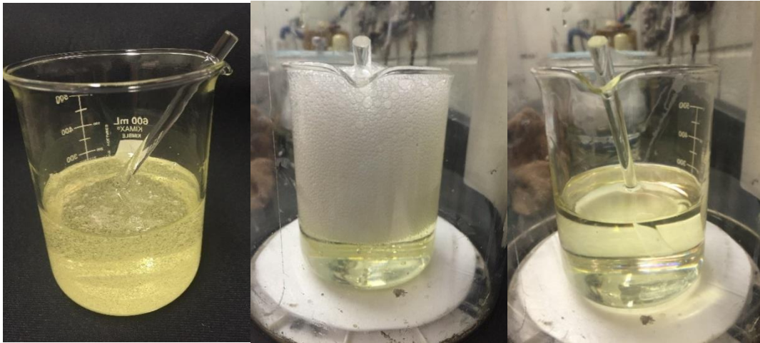
Figure 62. (left) Fuel mixture after mixing containing entrained air bubbles in atmosphere, (middle) fuel mixture containing entrained air bubbles under vacuum, and (right) fuel mixture containing no entrained air bubbles.
