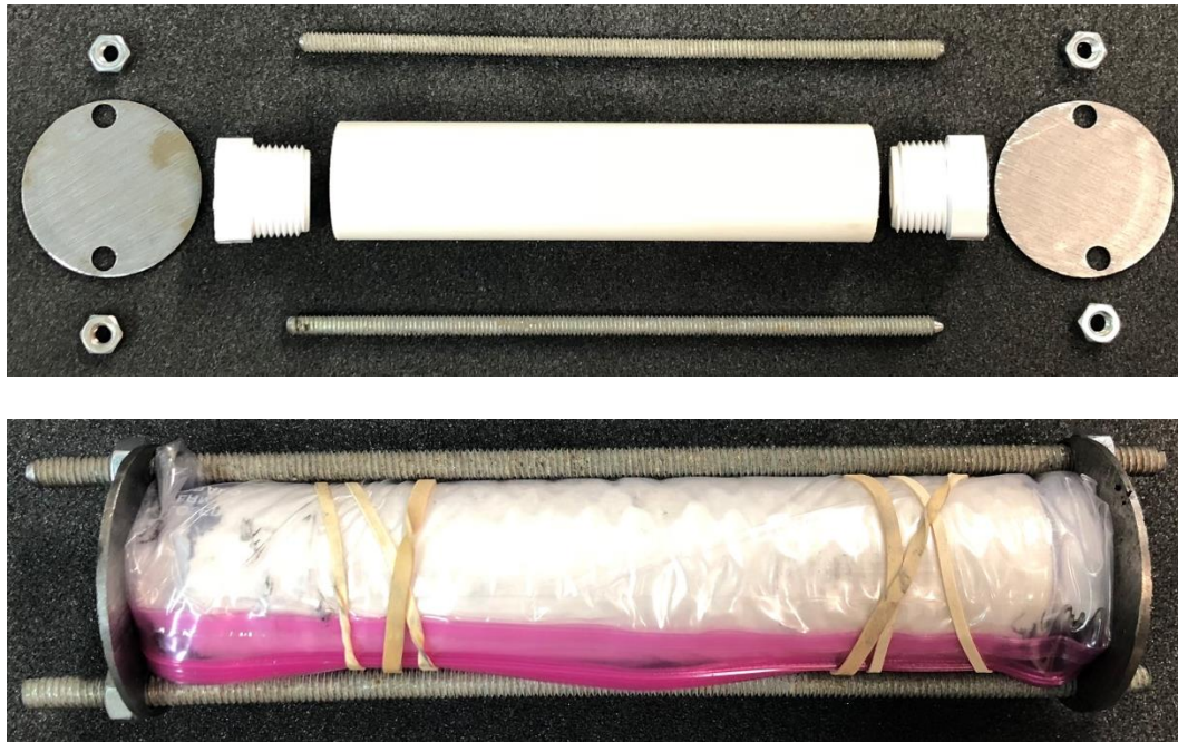
Figure 63. (top) Unassembled and (bottom) mold components for mixed-fuel (HTPB/paraffin) specimen.
