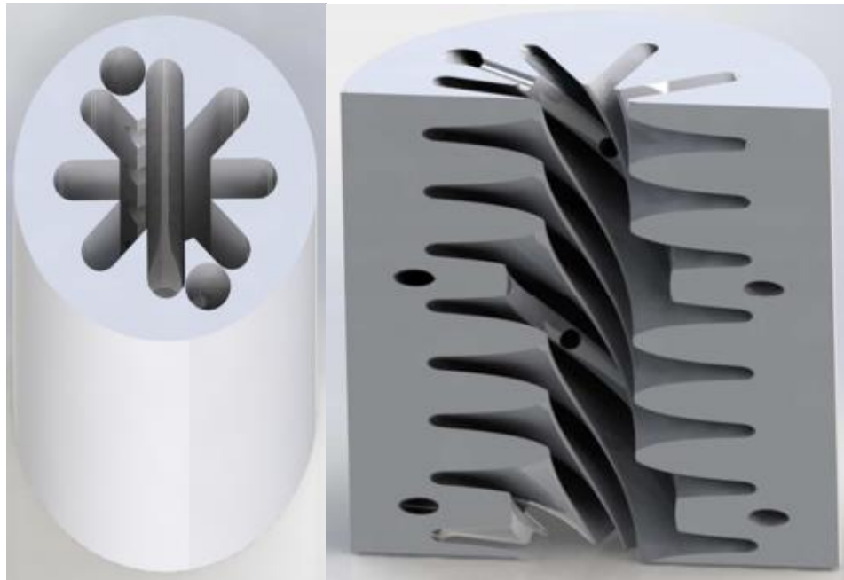
Figure 11. Fuel grain geometries manufactured with internal flow injection structures. Images taken from Ref. [222].
