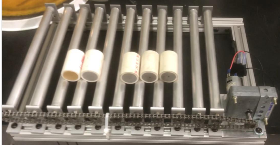
Figure 64. Roller assembly utilized to mitigate additive particle settling effects during fuel curing. Fully processed motors are shown.
