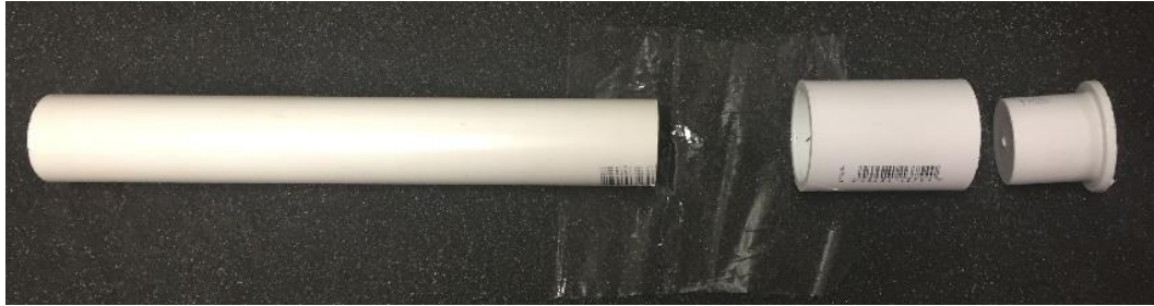
Figure 61. Unassembled mold components for baseline (plain HTPB) fuel specimen.
