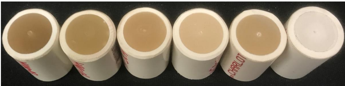
Figure 59. Representative mixed-fuel grains. (left to right) Plain HTPB, HTPB containing 0%, 10%, 25%, 50%, 75% paraffin, and plain paraffin.
