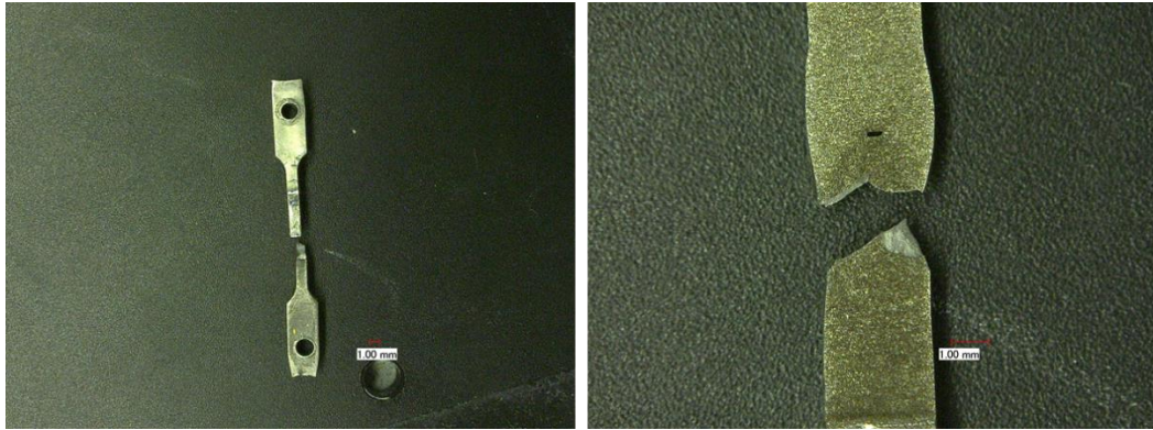
Figure 38- Ti-6Al-4V Bevel Welded To TiNb After Tension Test
