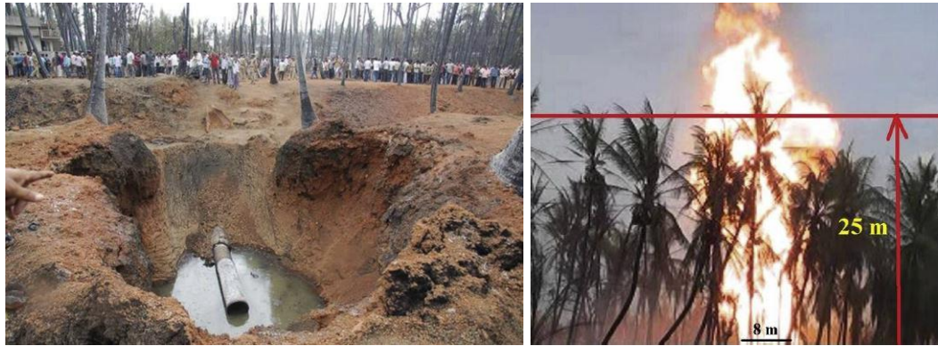
Figure 1 Resulting crater, pipeline full-bore rupture and fire, Andhra Pradesh, India Reprinted from [2]
