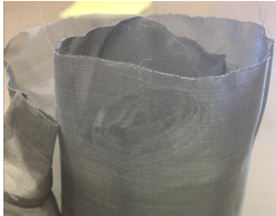
Figure 9: Image of Aluminum Wire Cloth. Material: Aluminum 5052, Mesh Size: 200×200, Porosity: 34%, Wire Diameter: 0.0021”.
