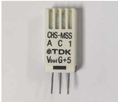
Figure 4-23 Relative humidity sensor.
