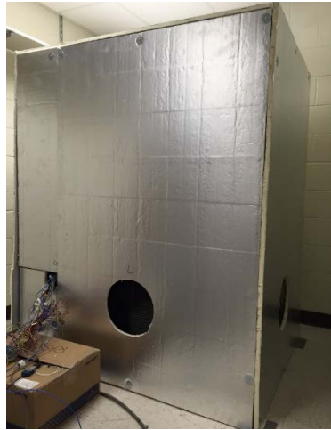
Figure 4-3 Insulation chamber for heating tests.
