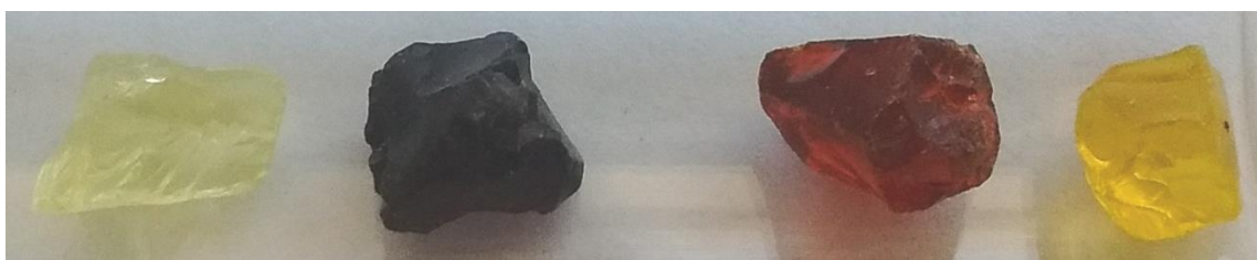
Figure 5.17 Silica specimens after absorbing the maximal amount of \text{Mo}(\text{CO})_6 , nickelocene, ferrocene, and cymantrene (left to right).
