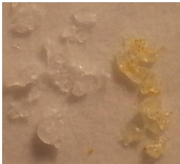
Figure 6.10 Comparison of pristine HDPE (left) and HDPE that has been exposed to 10 for one week.
