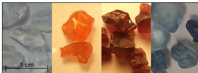
Figure 5.2 Large silica gel pieces. From left to right: virgin silica gel pieces, with adsorbed ferrocene ( 10a ), prepared and stored under N_2 , 10a after partial oxidation in air, and fully oxidized 10a (ferrocenium salt).
