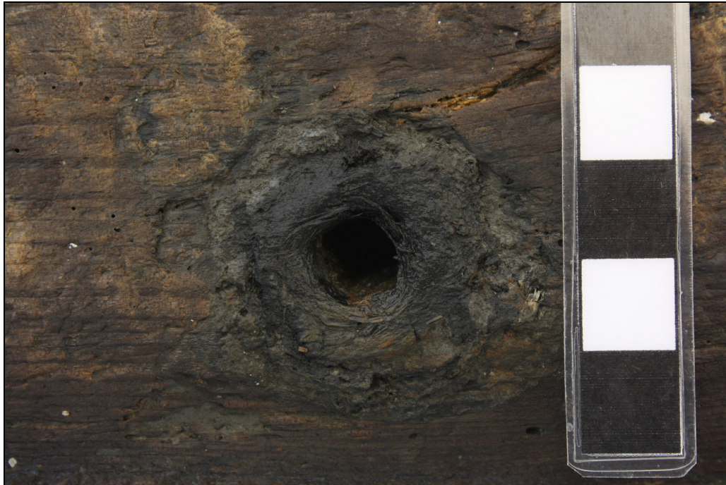
Figure 4.82. Nail on PS 5-1 outer face at FR 15. Note fibers that had been wrapped around the base of the nail shank.
