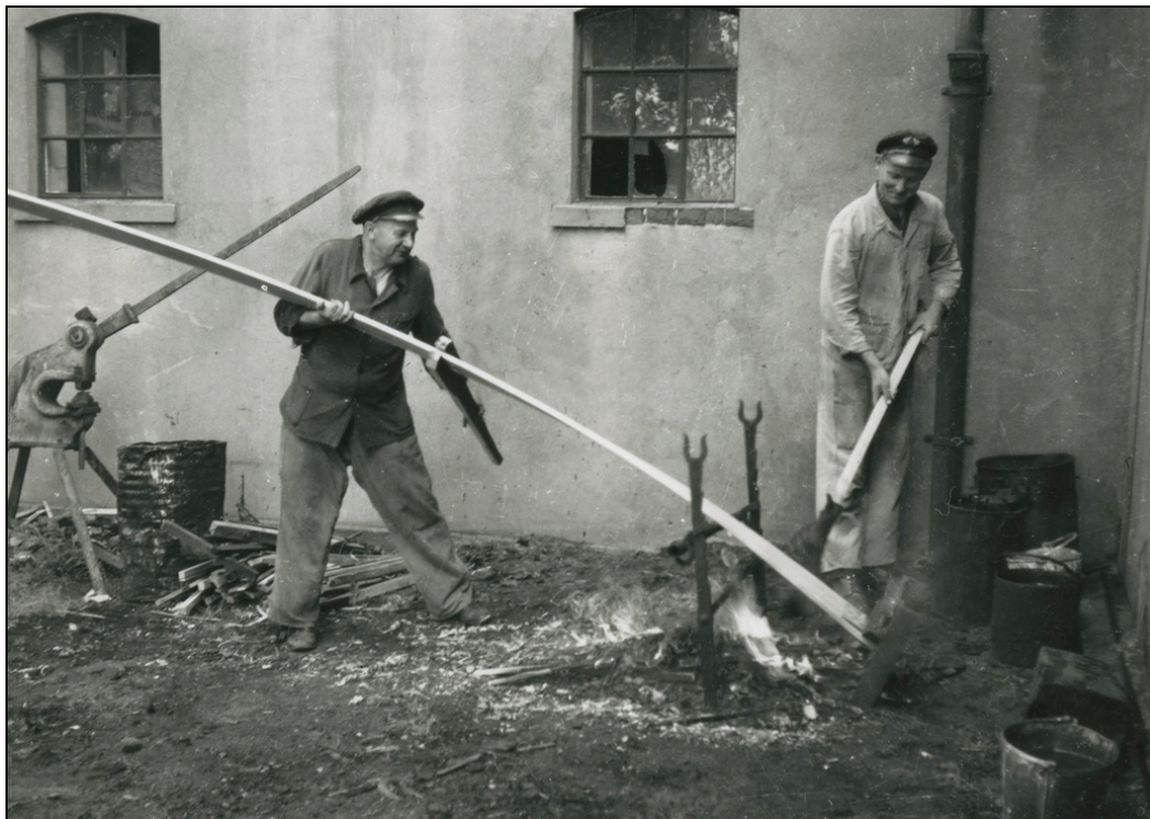
Figure 5.1. Workers char-bending a plank in an early 20 th -century shipyard along the Weser River in northern Germany. Photo Deutsches Schiffahrtsmuseum; used with permission.
