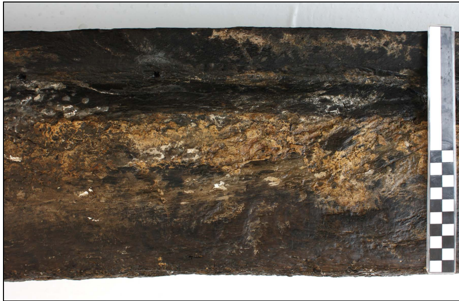
Figure 4.14. Pitch on Keel 2 port face, below rabbet.
