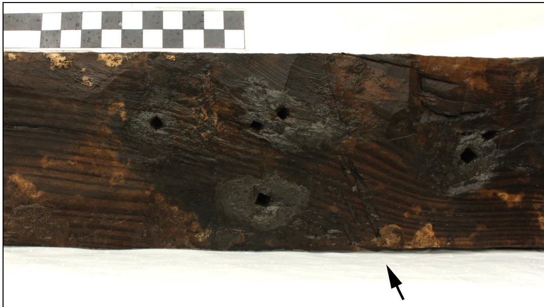
Figure 4.49. Cut marks on the outer face of FR 20.
