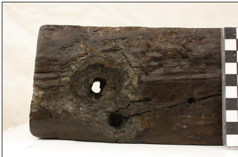
Figure 4.119. Sternson KS 1 inner face at forward end. Note bolt hole and secondary nail hole.
