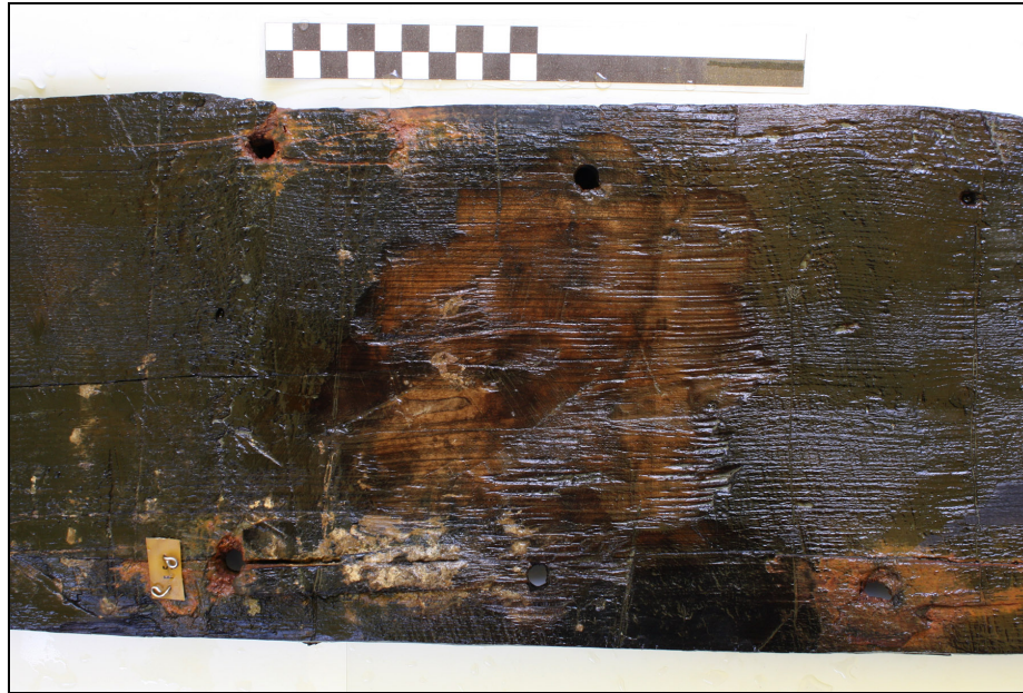
Figure 4.69. SS 8-1 at FR 5-FR 7. The charred inner face of the plank is adzed down at the original location of futtock F 5; note lighter color at adzed area.
