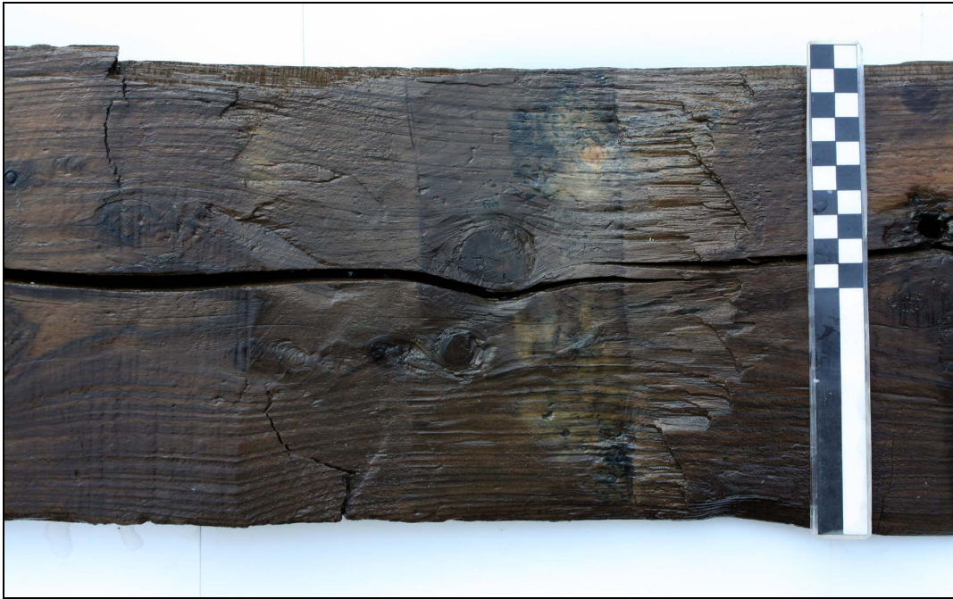
Figure 4.153. Roughly-adzed area on outer face of SC 2 at FR 12. Note pressure mark and pitch stain at frame location.
