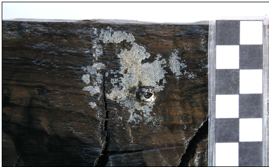
Figure 4.141. Marine growth and barnacle on the outer face of SST 1-2 at FR 14-FR 15.
