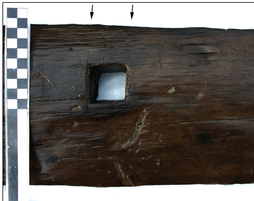
Figure 4.164. Mortise at S-Block 6 inner face. Note naturally rounded surface, score marks at mortise edges (arrows).
