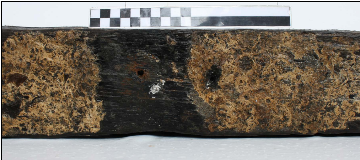
Figure 4.15. Thick pitch between frames on the Keel 2 inner face, with sparse patches under FR 19.
