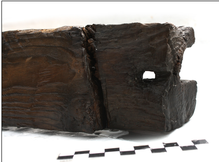
Figure 4.175. Notched outer face of BH FR 1 at sternson KS 1.
