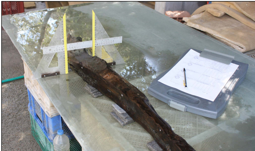
Figure 3.15. Sections were created with the aid of an adjustable, custom-made tool.
