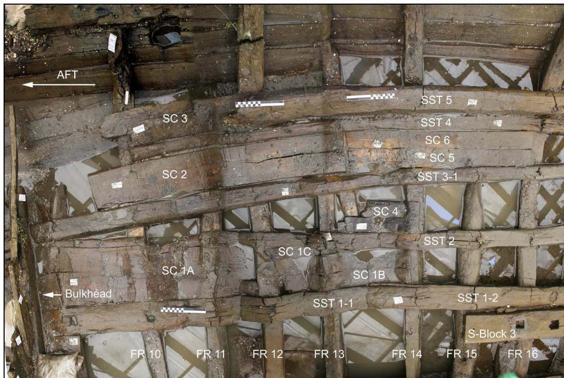
Figure 4.144. Photomosaic of port-side ceiling, forward of the bulkhead. SST 5 has slipped downward. Scale shown is 20 cm.
