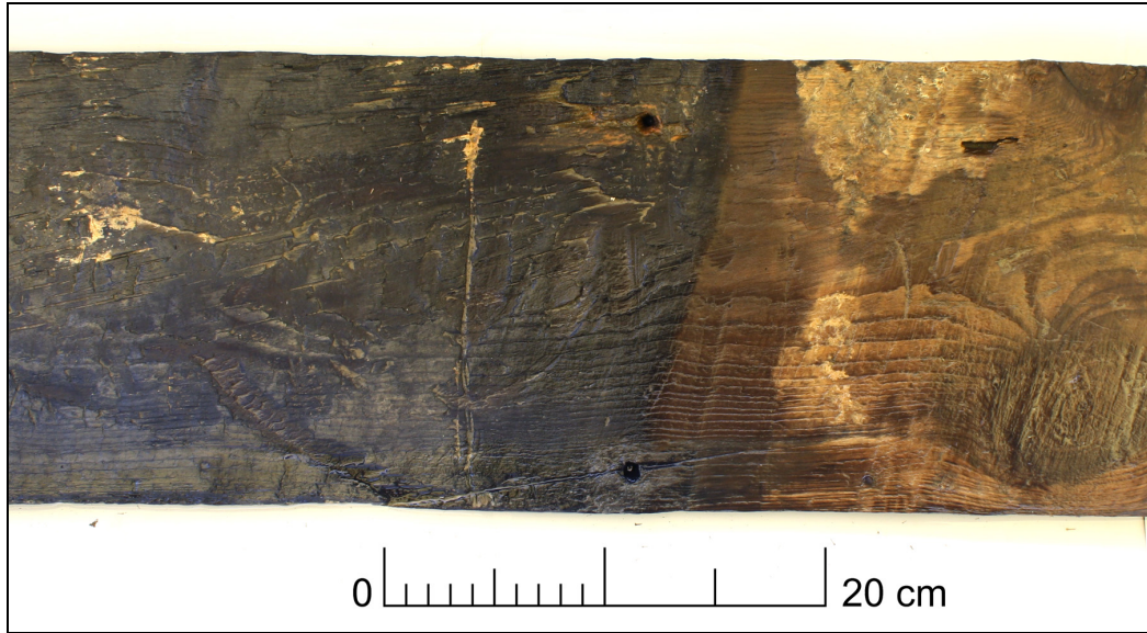
Figure 4.79. PS 3-2 inner face at FR 21. Note clearly-delineated charring and score marks at FR 21.
