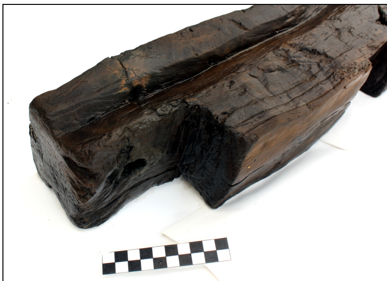
Figure 4.117. Forward end of sternson KS 1. Note rabbet from former use as a keel.
