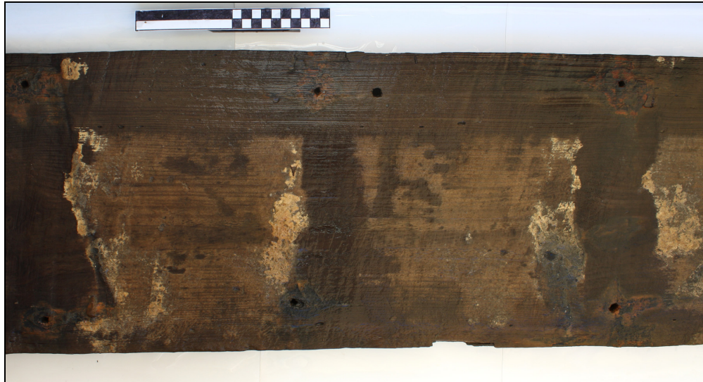
Figure 4.88. SS 2-3 inner face at FR 17-FR 19. Note pitch stain between frame stations and lack of pitch stain at SST 1 location (near upper edge).
