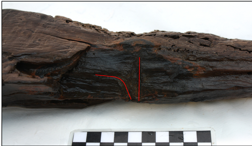
Figure 4.45. Traces of iron nails on the broken aft face of FR 25. Note straight nail next to a nail which bent upon insertion (red line added for clarification.)
