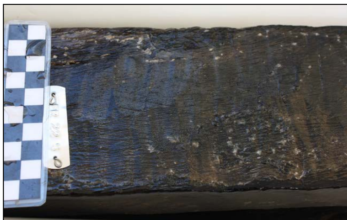
Figure 4.9. Adze marks on the inner face of Keel 3 at FR 21-FR 22.
