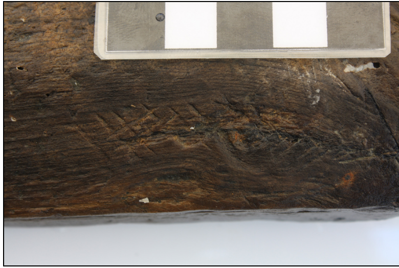
Figure 4.96. Small cuts across a grain defect on the outer face of PS 5-1 at FR 14.
