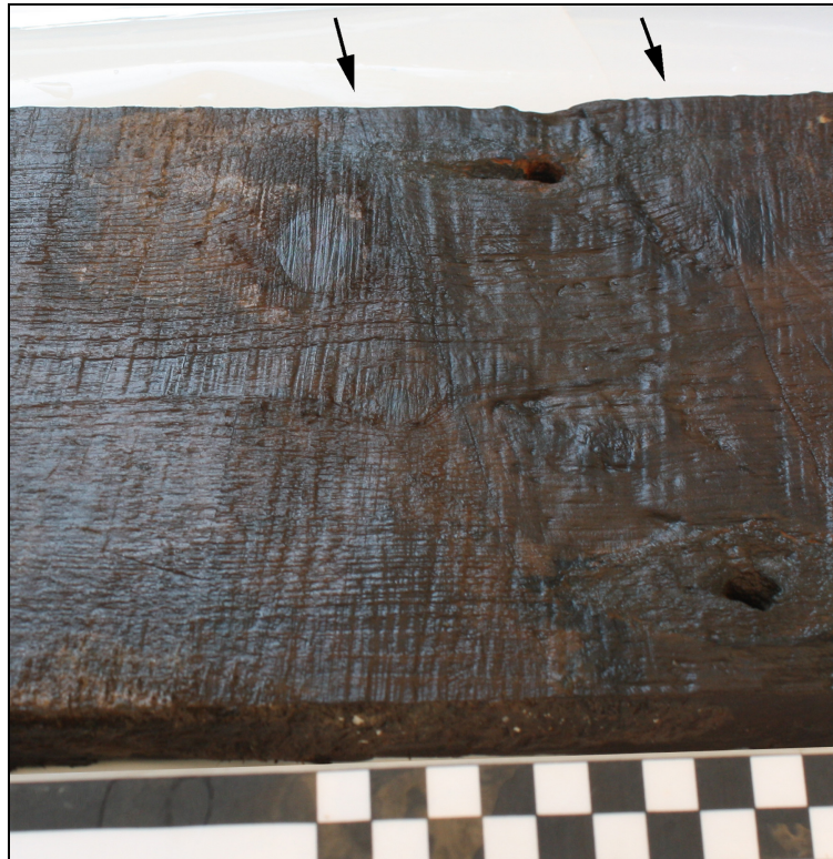
Figure 4.67. Score marks on PS 3-3 at FR 21. Differentiating between saw marks and score or other cut marks was facilitated through the use of raking light. Score marks here are denoted by arrows.
