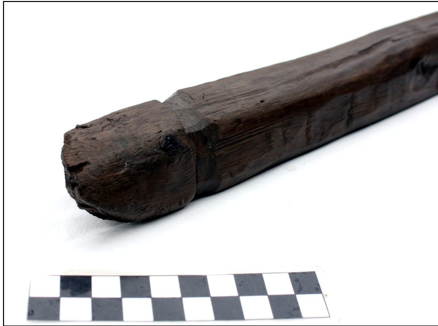
Figure 4.180. Whittled collar near broken end of UM 21.
