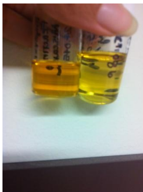
Figure 11. Initial Bio-oil Distillate Color. This figure shows the color of the bio-oil distilled fractions immediately after distillation. Initially, most fractions ranged from light yellow to light orange in color.
