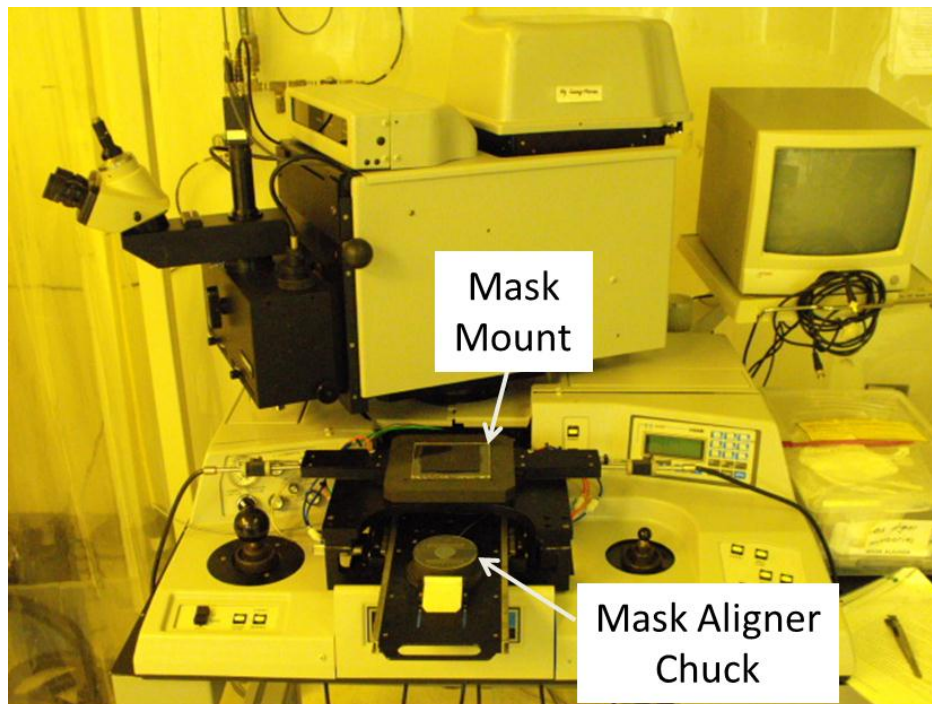
Fig. 2.8 Mask aligner with mask and wafer in place (UV light turned to side)
