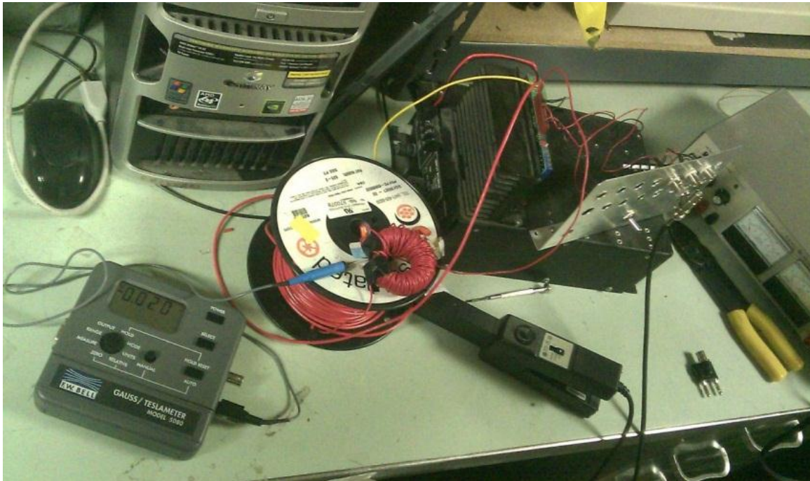
Fig. 3.6 Experimental Setup to Retrieve 4340 BH Curve
