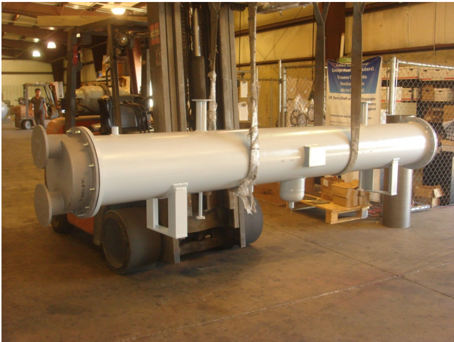
Fig. 2.10: Fabricated SX Chiller for Norwegian Test Stand
