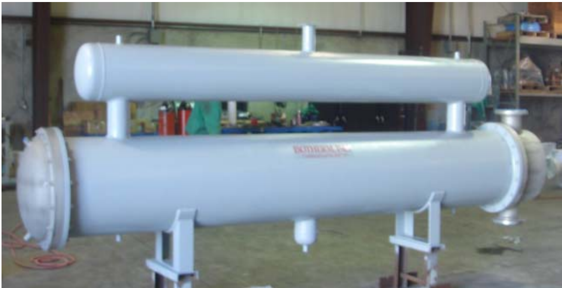
Fig. 6.1: Flooded Evaporator for Cheese Plant
