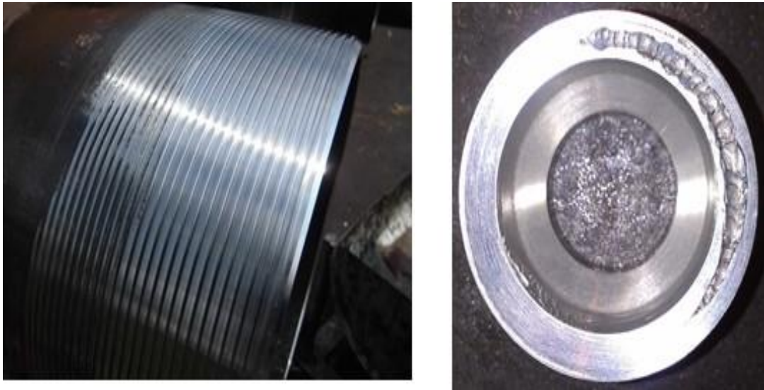
Figure 15. Examples of galling damage on tubing threads and on a flat disc shaped metal specimen.
