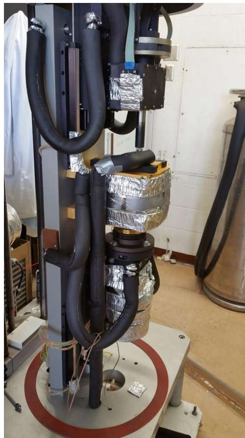
Figure 11. High temperature tribometer (HTT) modified to accept liquid nitrogen for low temperature experiments.
