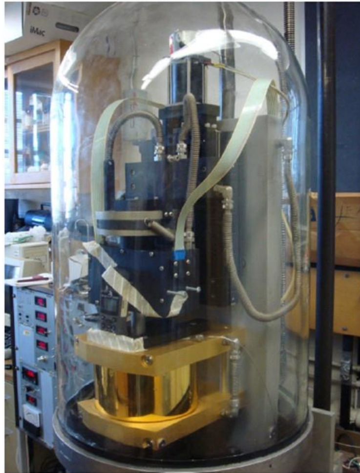
Figure 5. Image of the high temperature tribometer (HTT) apparatus used in this research.
