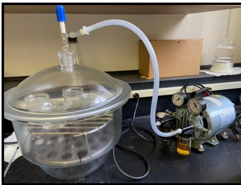
Figure 6 The vacuum impregnation system used in this study.
