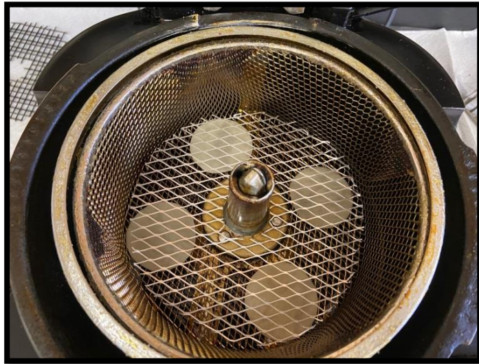
Figure 7 Samples loaded in the deep-fat fryer basket.
