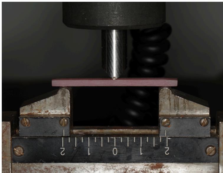
Figure 2. Three-point Flexural Test Setup
