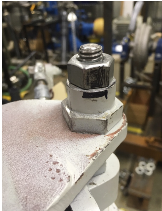
Figure 13: Governor Valve Linkages with Attached Stem Positioning Nut and Positioning Nut Indicators
