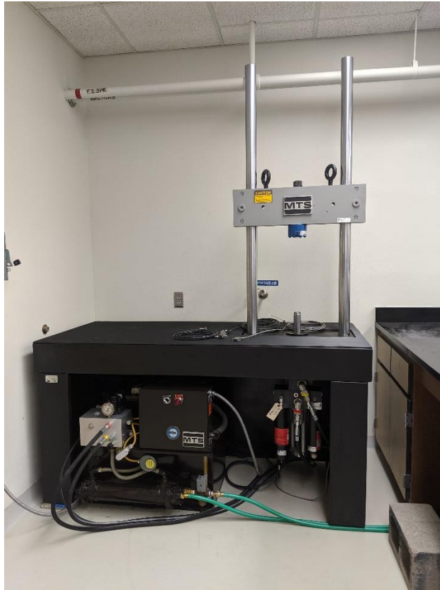
Figure 26: MTS fatigue testing machine in Ocean Engineering Materials and Structural Lab
