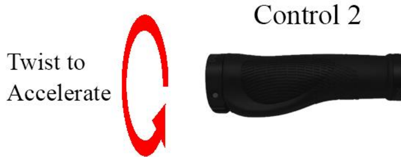
Figure 5.8: Throttle to control bicycle torque
