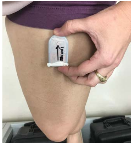
Figure C-3 Placement of the activPAL ™
