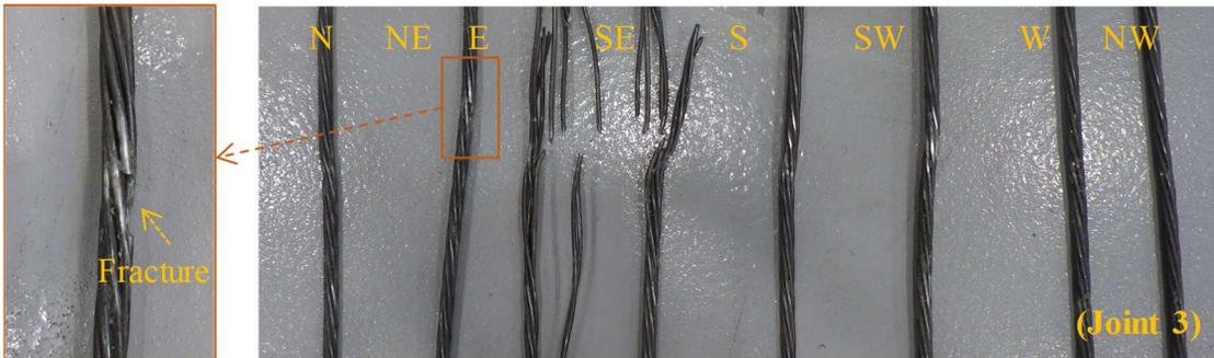
Figure 4-328. Phase III, final damage inspection: posttensioning tendons
