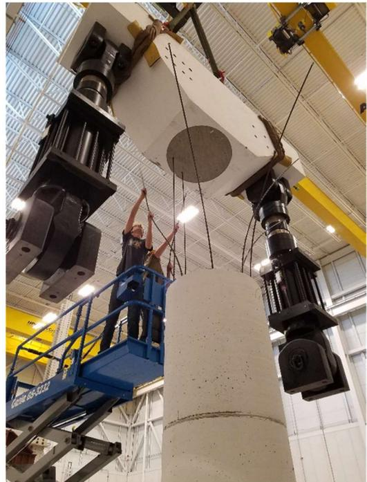
**Figure 4-42. Moving loading beam and placing it on column**
