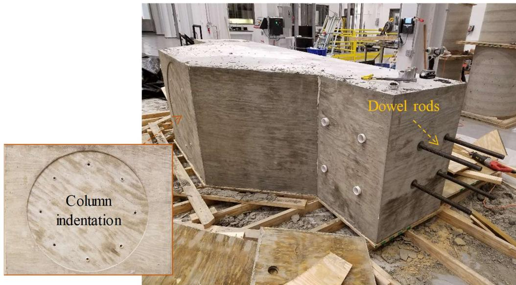
**Figure 4-31. Loading beam after form removal**
