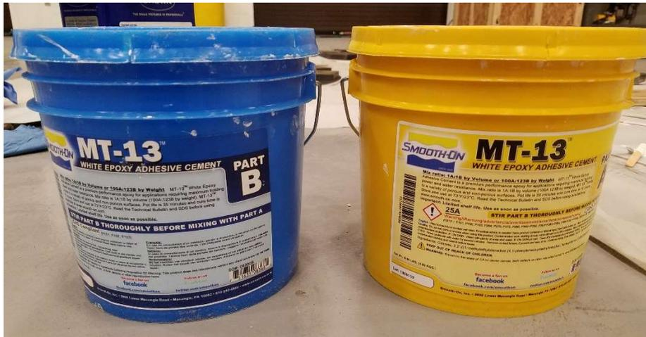
**Figure D-1. Epoxy product used for bonding sliding joint interface materials to column segment end surfaces**
