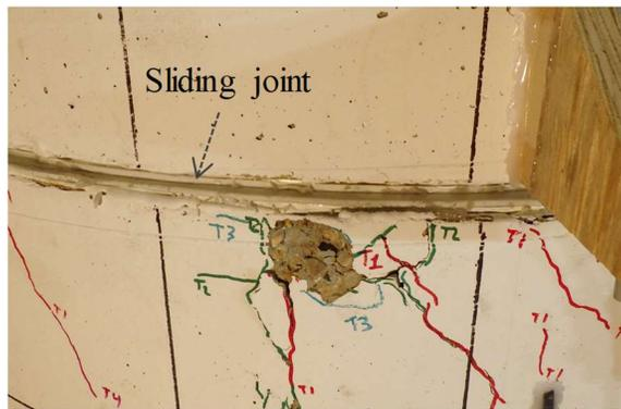
Figure 4-104. Phase I, Loading Set 3: spalled concrete below Joint 2 on west side
