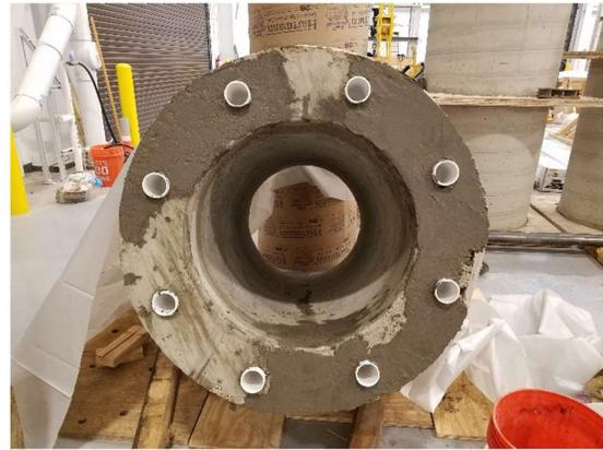
**Figure C-5. Repaired top column segment**
