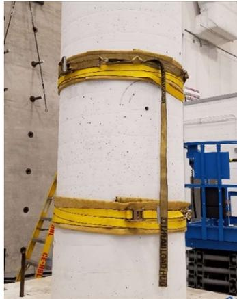
**Figure 4-253. Prevention of accidental sliding at sliding joints using ratchet straps**
