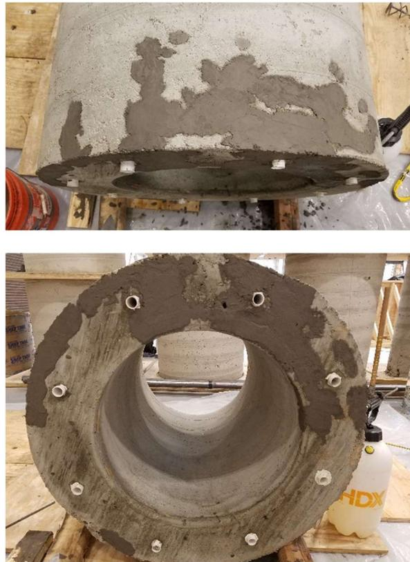
Figure C-4. Repaired bottom column segment
