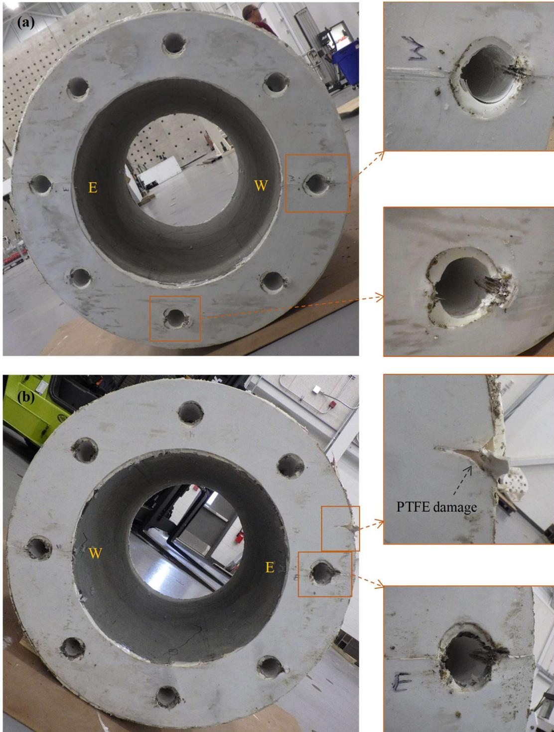
Figure 4-325. Phase III, final damage inspection, middle segment: (a) bottom end;
