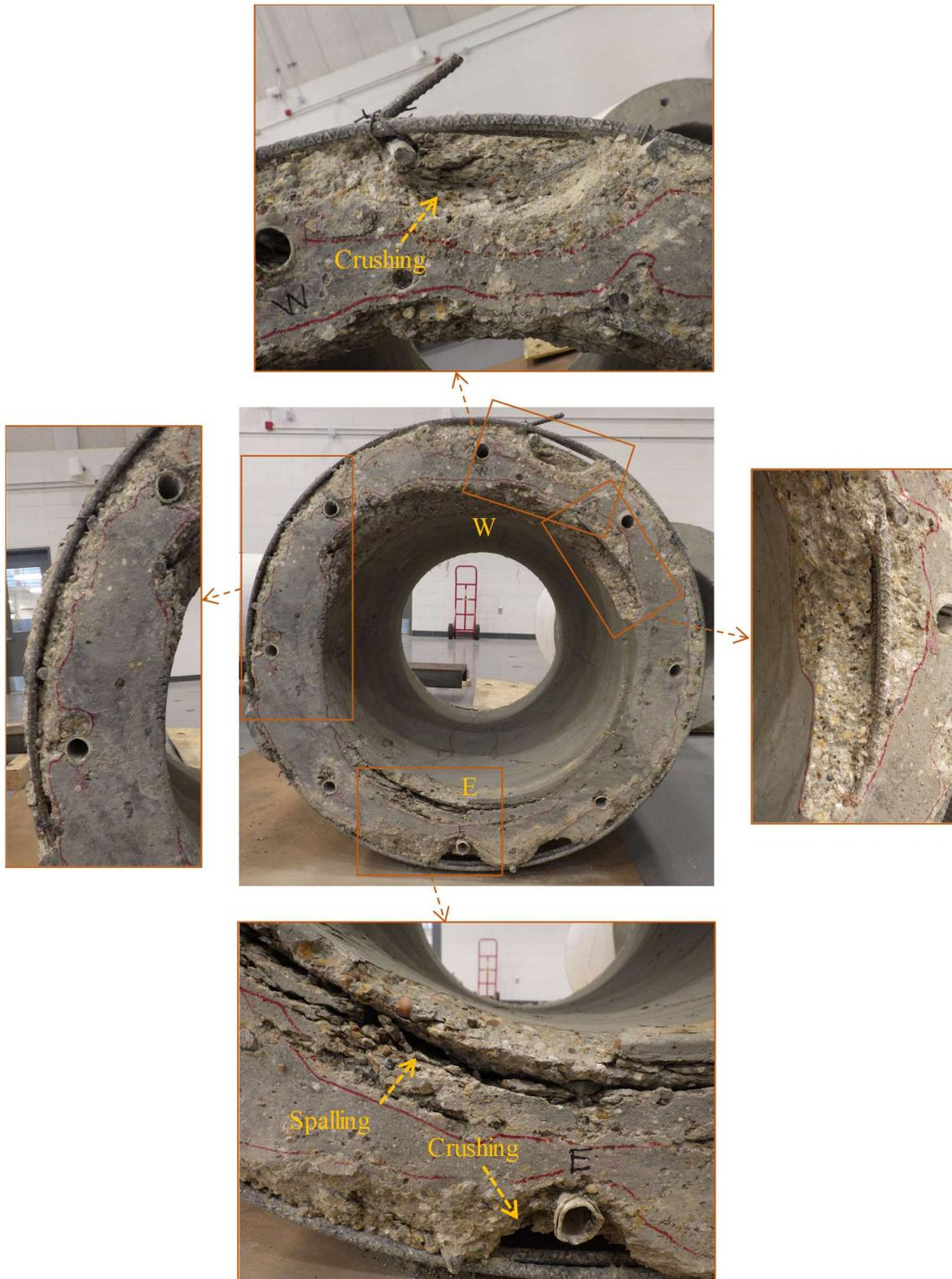
Figure 4-243. Phase II, final damage inspection: bottom surface of bottom segment
