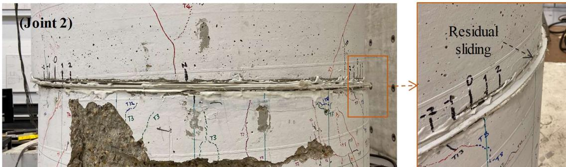
**Figure 4-411. Phase IV, final damage inspection: residual joint sliding**
