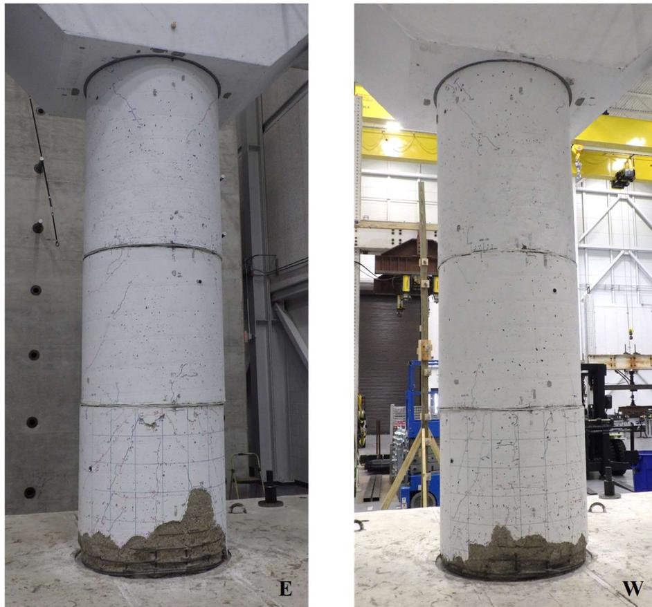
**Figure 4-237. Phase II, final damage inspection: east and west sides of column**
