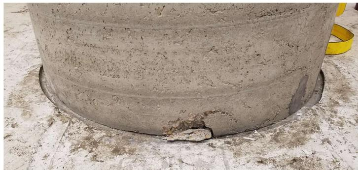
**Figure 4-141. Bottom column segment damage caused during test setup assembly**
