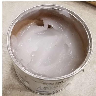
**Figure D-2. Grease product used to cover sliding joint surfaces**
