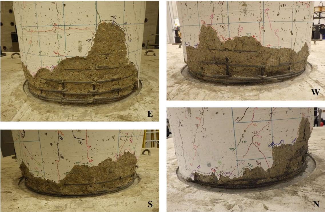
**Figure 4-238. Phase II, final damage inspection: concrete damage around bottom rocking joint**
