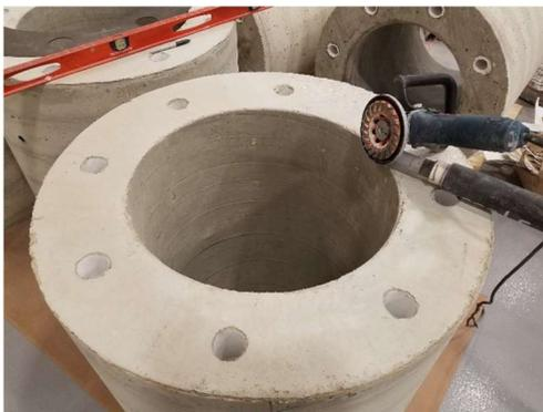
**(1) Grinding and removing dust by compressed air**
