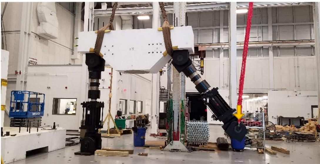
**Figure 4-252. Lifting of loading beam before its placement on column**
