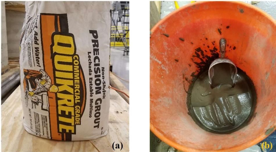
Figure C-3. (a) Grout product used for repair; (b) flowability of mixed grout
