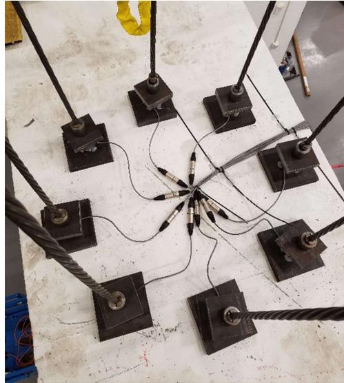
**Figure 4-44. Tendon anchors and load cells above loading beam**
