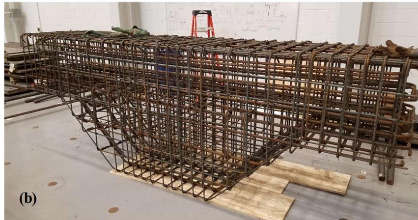
**Figure 4-27. Steel cage for loading beam: (a) assembly; (b) completed cage**
