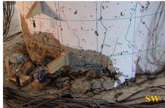
Figure 4-228. Phase II, loading protocol HSR2\_TU\_CNT\_S6\_DR\_8: concrete damage on bottom segment
