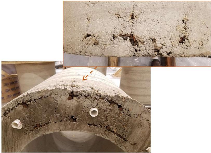
**Figure C-1. Bottom segment of column tested in Phase II after formwork removal**
