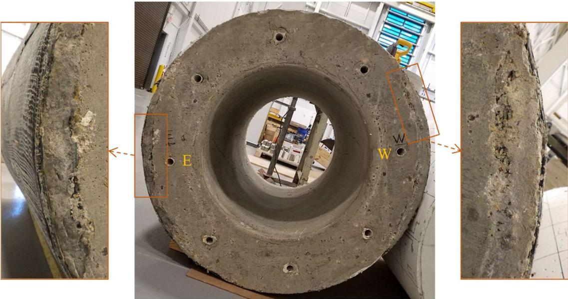
**Figure 4-133. Phase I, final damage inspection: bottom surface of bottom segment**
