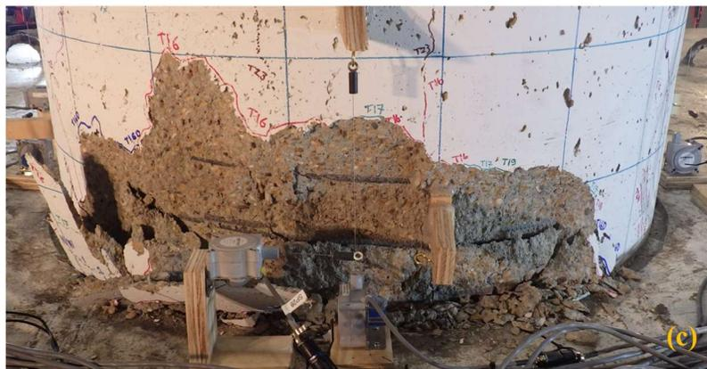
**Figure 4-197. Phase II, Loading Set 4, concrete spalling near west segment toe after tests under loading protocols: (a) HSR2\_TU\_CNT\_S4\_DR\_4\_T2D\_0\_5; (b) HSR2\_TU\_CNT\_S4\_DR\_4\_T2D\_1; (c) HSR2\_TU\_CNT\_S4\_DR\_4\_T2D\_2**
