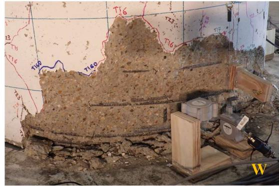
**Figure 4-218. Phase II, loading protocol HSR2\_TU\_CNT\_S6\_DR\_6: concrete damage on east and west sides of bottom segment**
