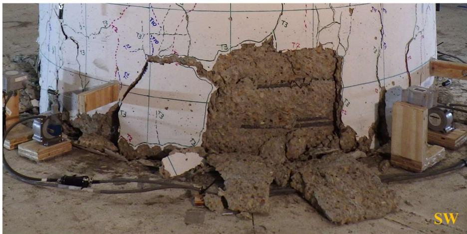
**Figure 4-397. Phase IV, Loading Set 3: damage spread above bottom rocking joint**
