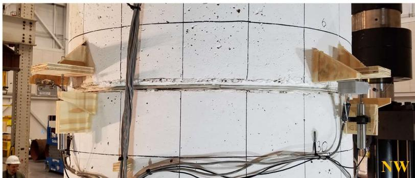
**Figure 4-61. Phase I, initial state of second sliding joint (Joint 3)**
