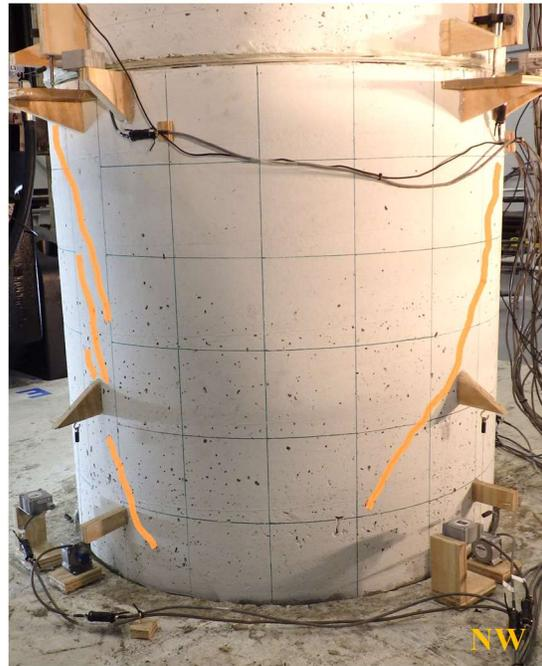
**Figure 4-260. Phase III, initial vertical load application: hairline cracks on bottom column segment**
