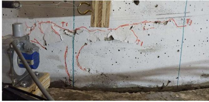
**Figure 4-354. Phase IV, loading protocol HSR3\_BI\_CNT\_S1\_DR\_1\_3: slight spalling near south quadrant of bottom rocking joint**
