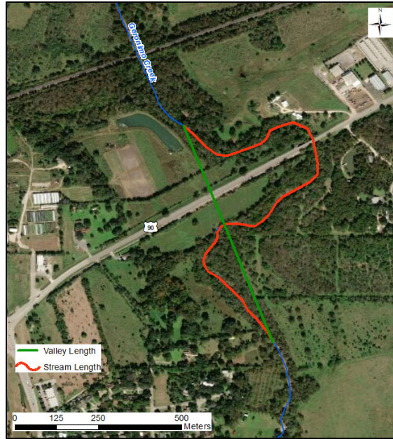
Figure 4.4 Stream length and valley length shown for a section that includes the study site within Geronimo Creek in Seguin, TX.
