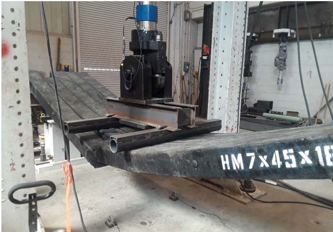
Figure 5 Photographic documentation of experimental four-point bend test, post-failure
