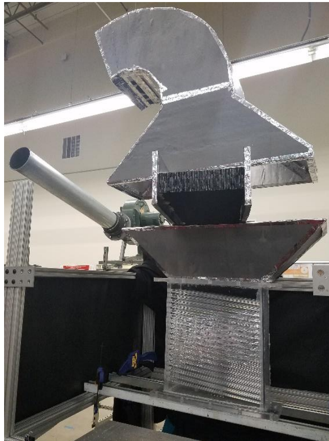
Figure 12. Honeycomb placement inside wind tunnel
