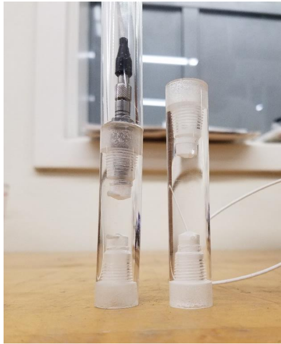
Figure 20. Dynamic pressure transducer fitted inside of a hollow acrylic rod
