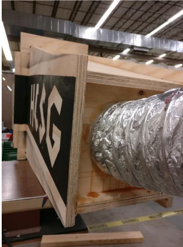
Figure 13. Wooden outlet connected to blower and aluminum duct
