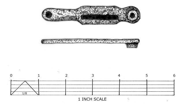
**Figure 47. Trigger Plate**
