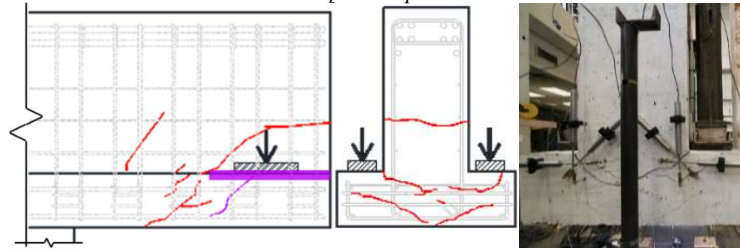
(a) LD reference (Pre-retrofit) specimen (T5E1) showing side elevation and end views of cracked condition with photo at end of test.
