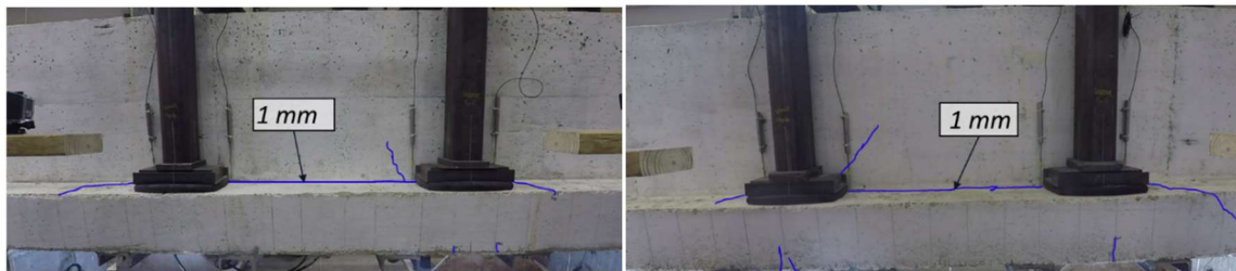
(c) Hanger-deficient 2-PT threadbar (T811)
