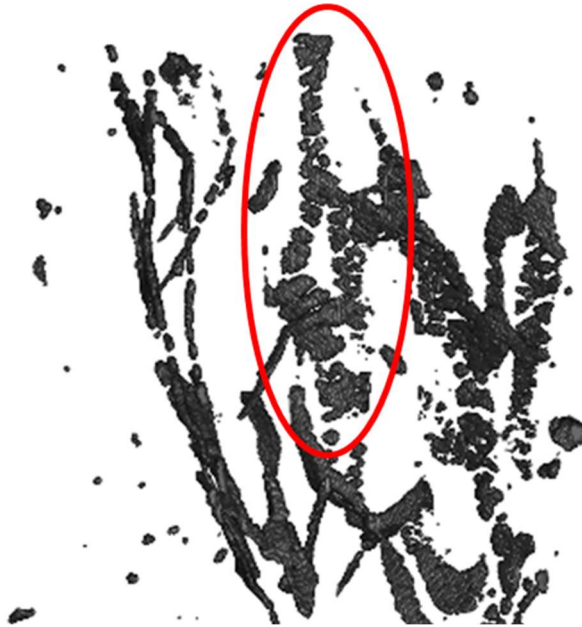
Figure 40: Small particles forming long stringers in rolled AZ31B
