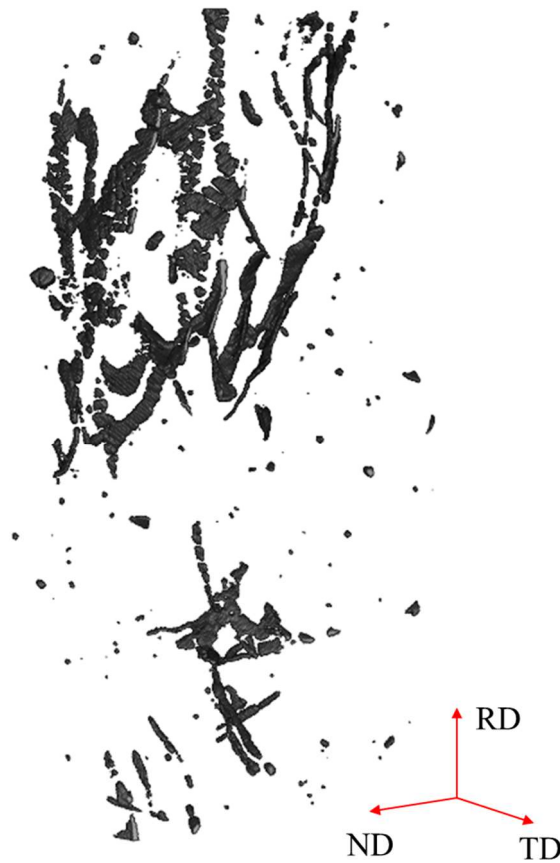
Figure 29: Rolled AZ31B microstructure showing second phase particles
